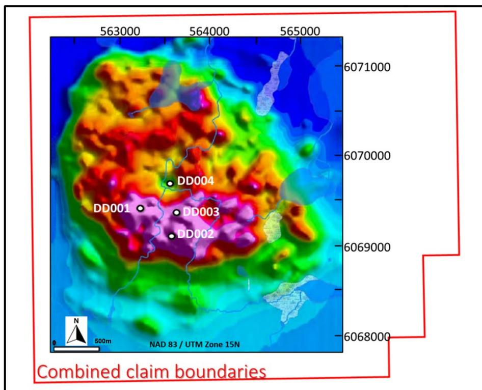
Figure 3. Aeromagnetic TMI of large circular carbonatite with variation in the magnetics showing partial ring structures with a magnetic low in the centre extending to the north-eastern margin of the intrusive.
