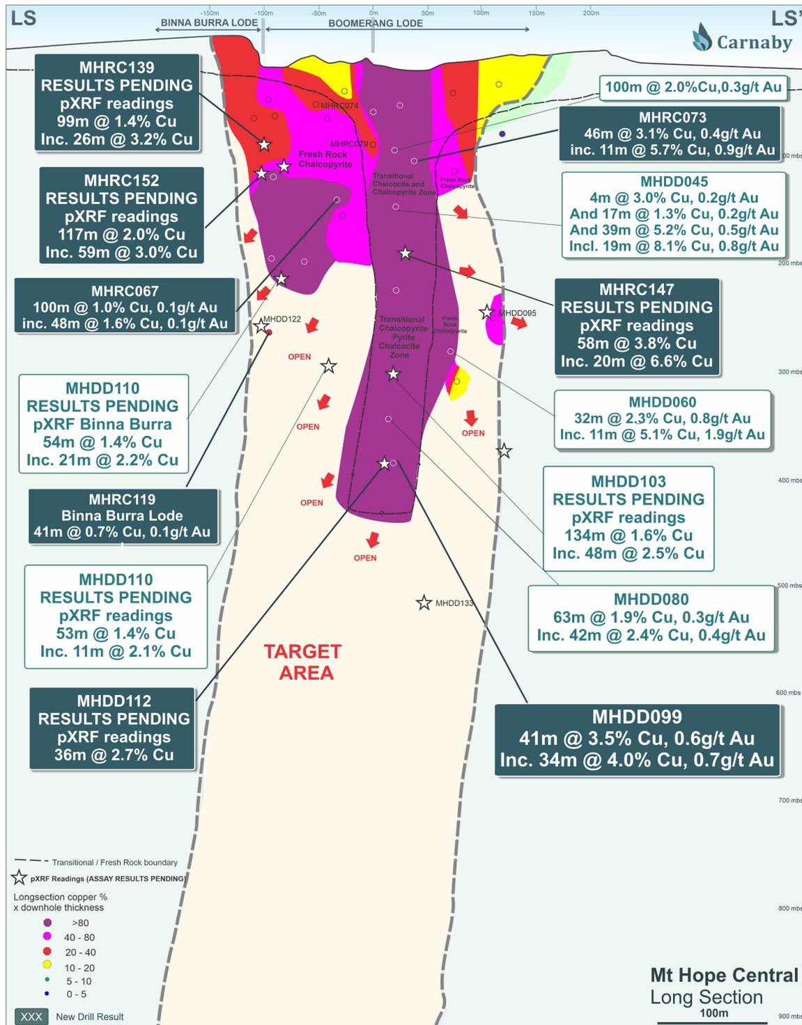
Figure 4. Mount Hope Central Boomerang Lode Long Section.
