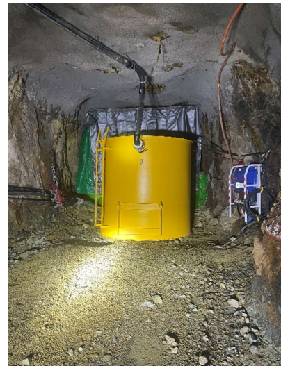
Figure 1: Underground portal, secondary ventilation fan installation and pumping at Mineral Hill underground.
