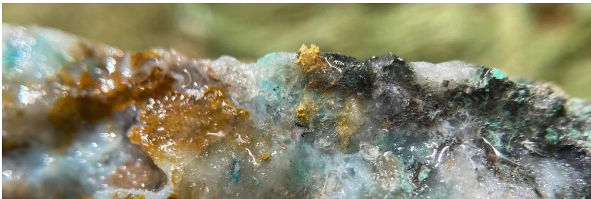
Figure 4: Image of visible gold within a quartz vein with secondary oxides and carbonates after sulphides from a mullock sample at the Lead Gold Mine (M09/091). The field of view is ~6cm. See Figure 6 at rear of JORC table for scale, location of collection and picture of entire rock chip.
