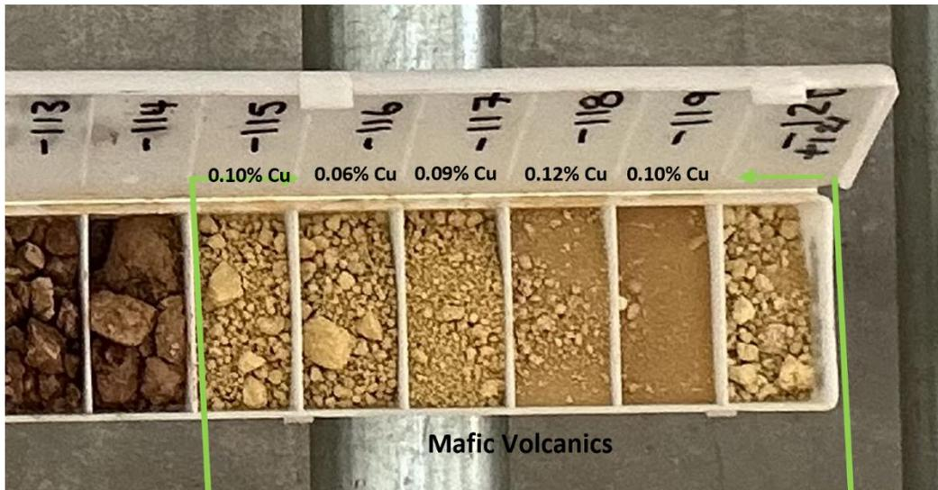
Figure 5. RC Chips from EHRC004, the last 5m are in mafic volcanics with low grade Cu mineralisation.
