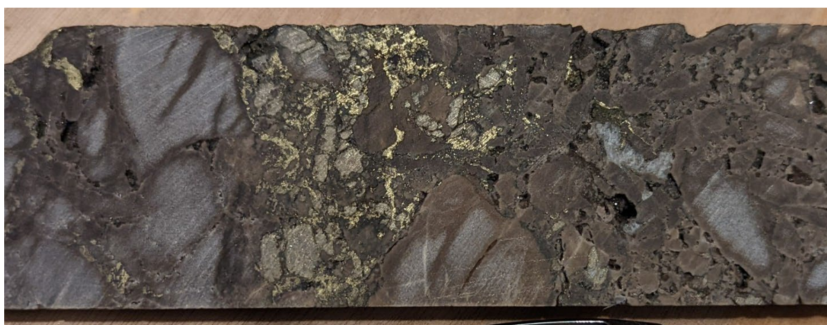
Figure 7: Chalcopryite (copper sulphide), pyrite (iron sulphide), sphalerite (zinc sulphide) and galena (lead sulphide) within vuggy bituminous dolostone in ST22-10 drill core from 313m downhole.
