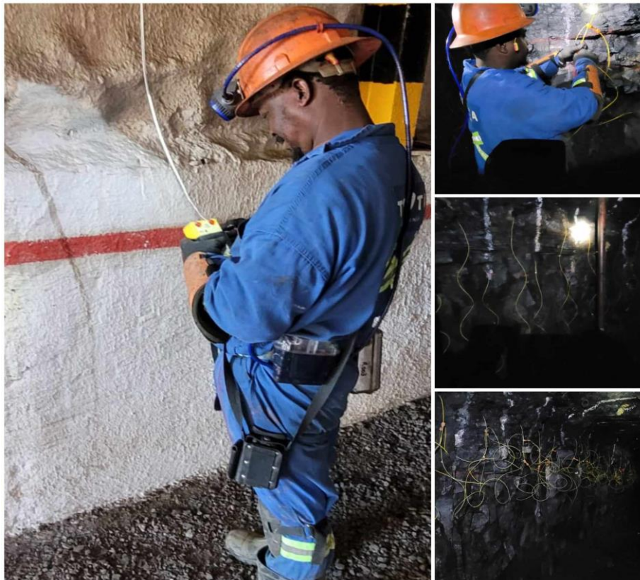
Figure 1: Drill and blast activity underway at Frankfort Gold Mine
