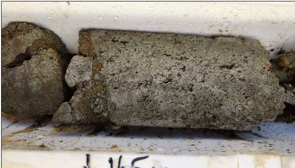
MLJDD018_164.5m_Massive pyrite in Breccia
