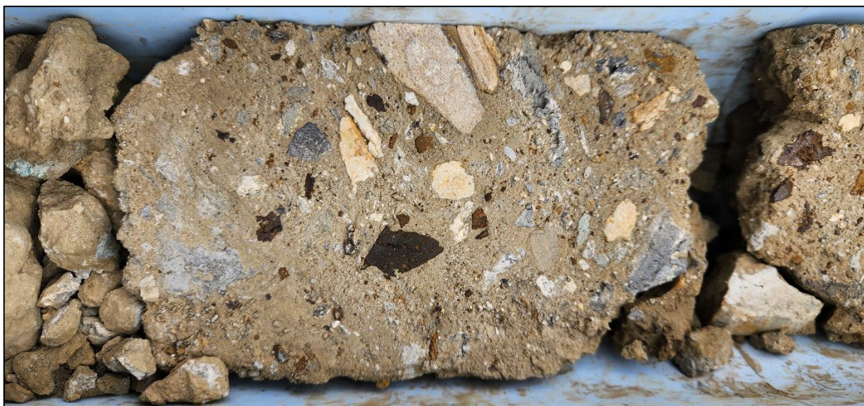
MLJDD020_178.0m_Polymictic Breccia with silica-pyrite clast
