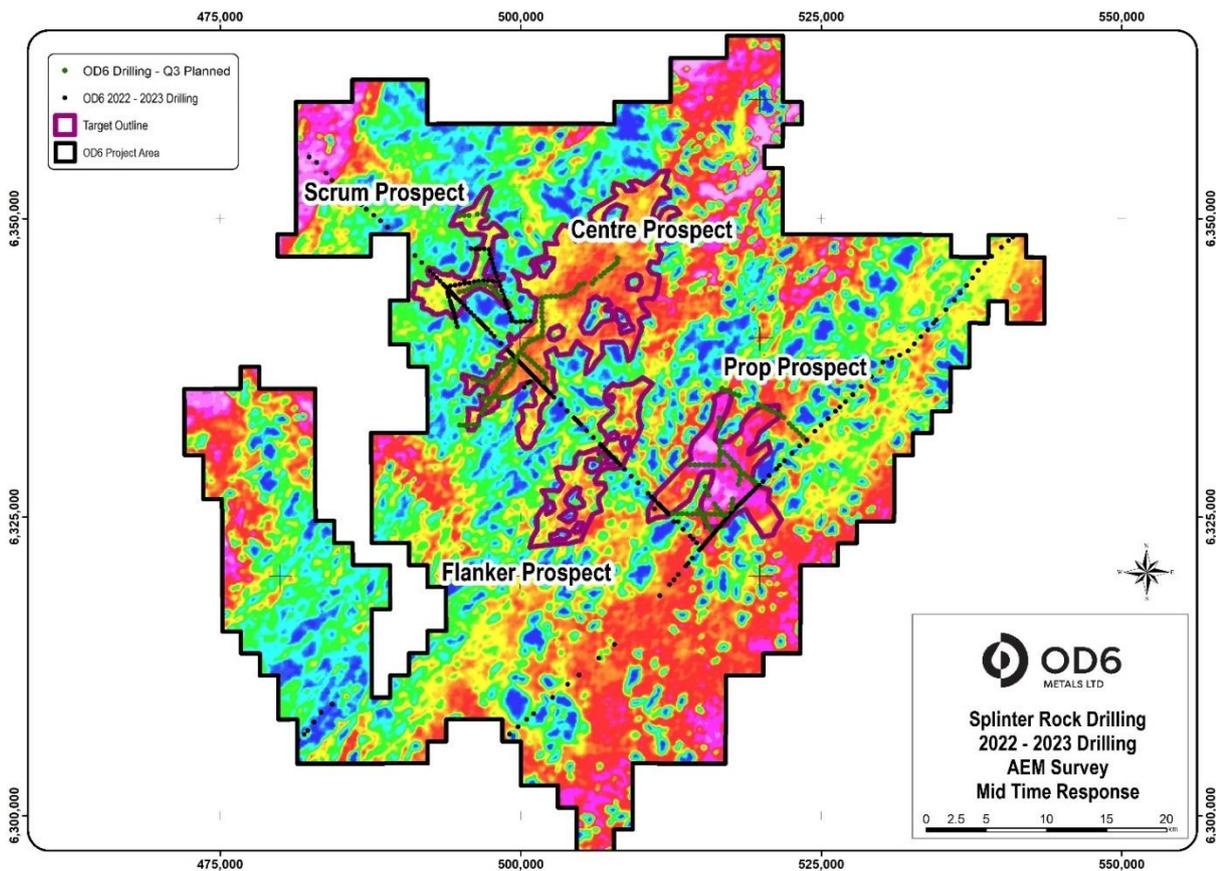
**Figure 8: AEM Mid time electromagnetic conductivity model of Splinter Rock project with drilling locations. Yellow, red, pink areas interpreted to indicated thicker clay zones, with blue areas the granites**
