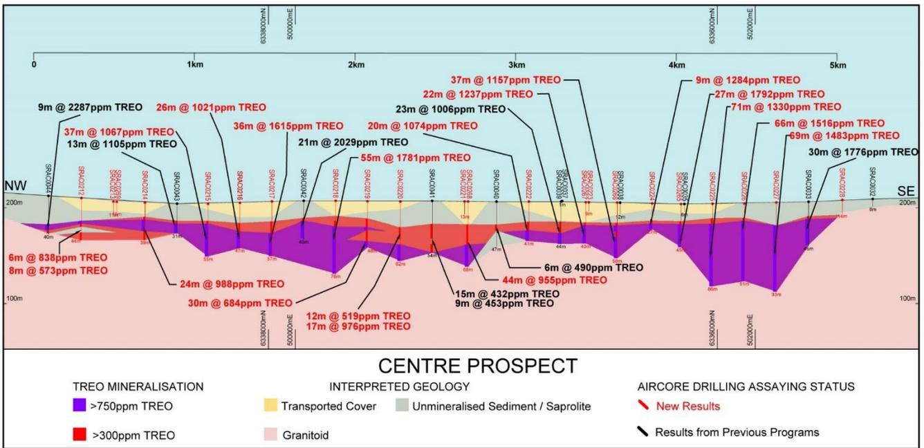
Figure 4: Centre Prospect Cross Section (vertical exaggeration x6)
