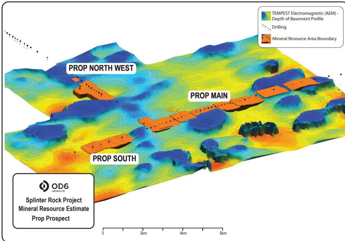
Figure 12: Prop Mineral Resource interpolation. Oblique view to the north.
