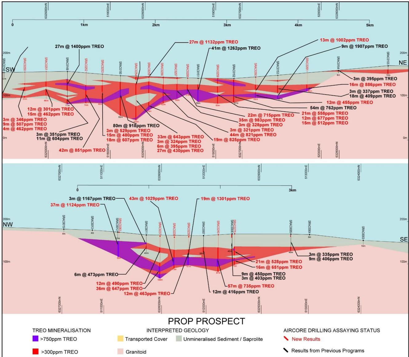
Figure 7: Prop Prospect. Upper image cross Section SW to NE along Parmango Rd drill line. Lower image Cross Section NW to SE (vertical exaggeration x6)
