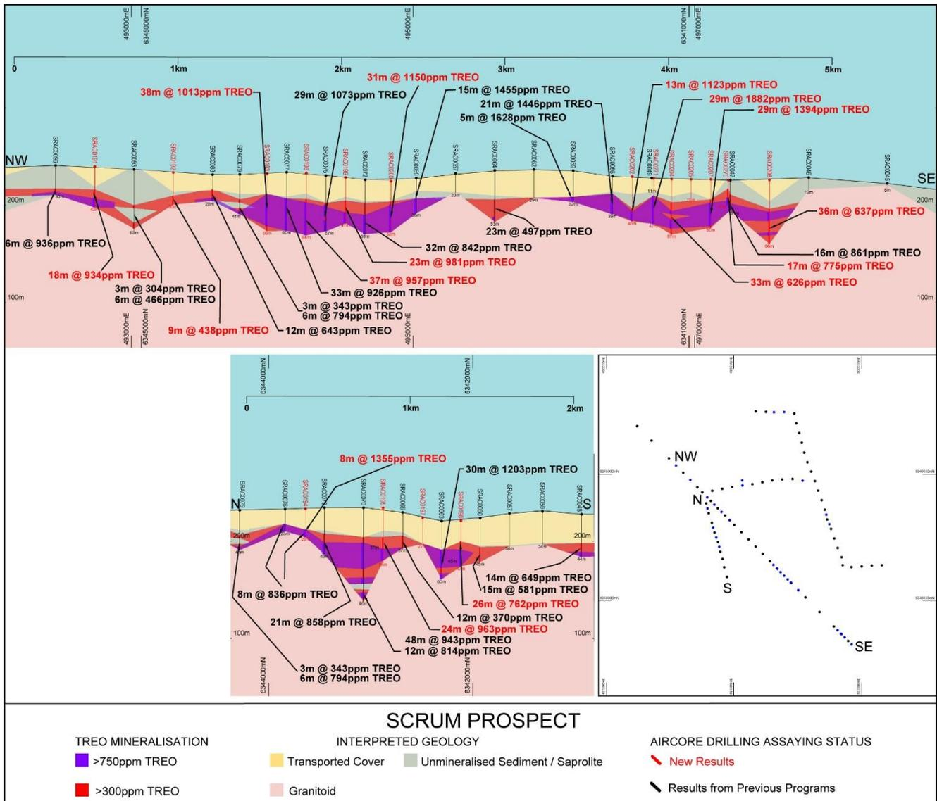
Figure 5: Scrum Prospect Cross Section (vertical exaggeration x6)
