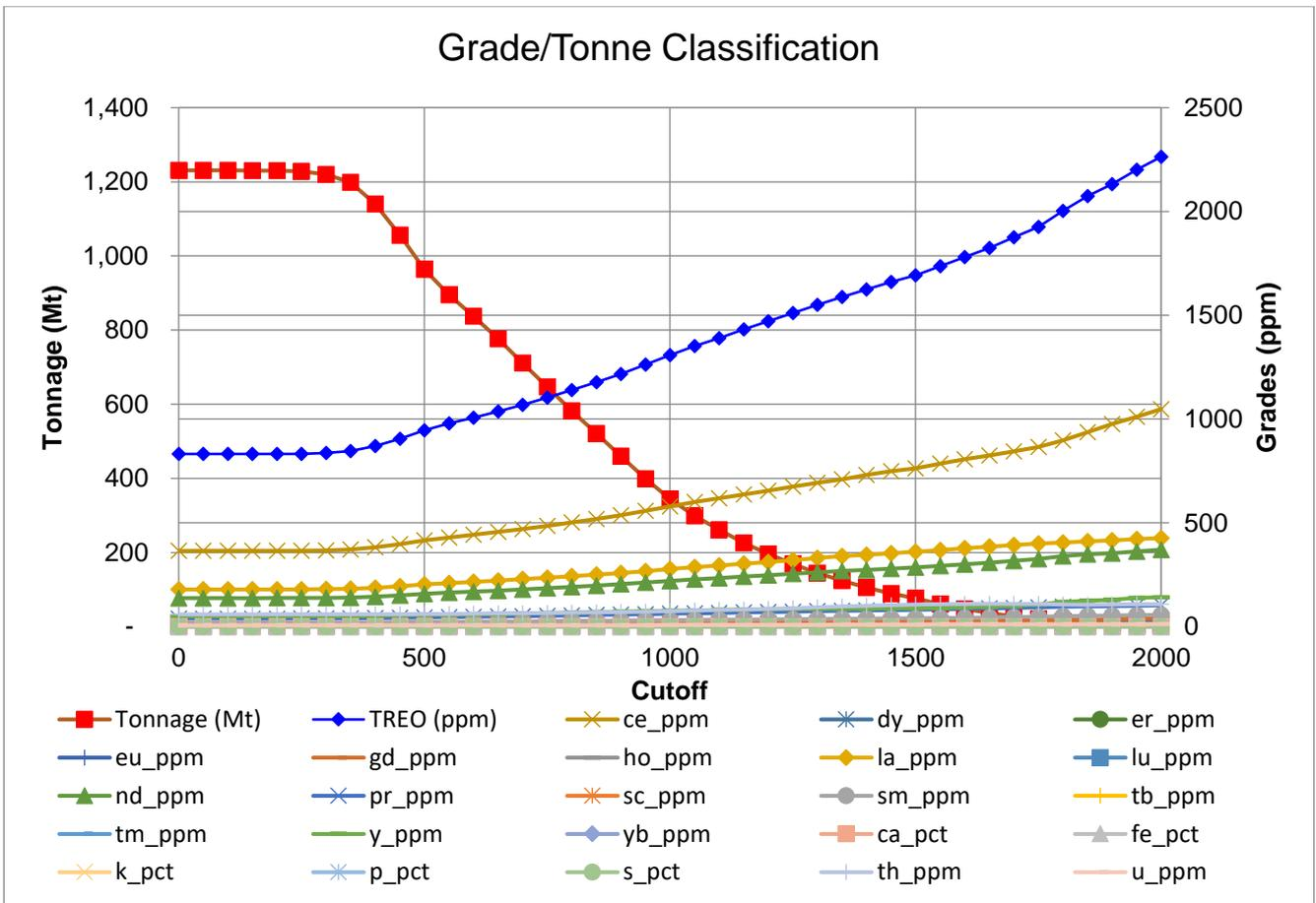
Figure 13: Splinter Rock Rare Earth project Tonnage and Grade Curve
