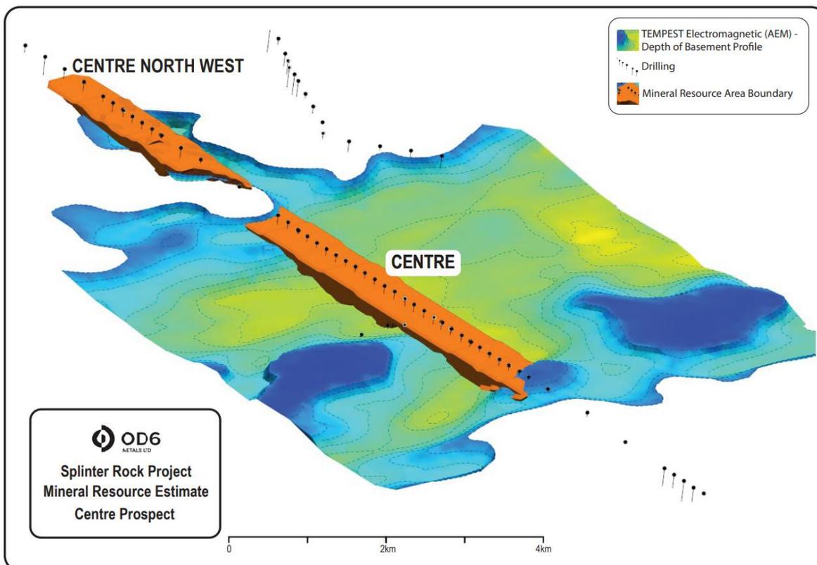
Figure 9: Centre Mineral Resource wireframe on the basement model (from AEM data). Oblique view to the north.
