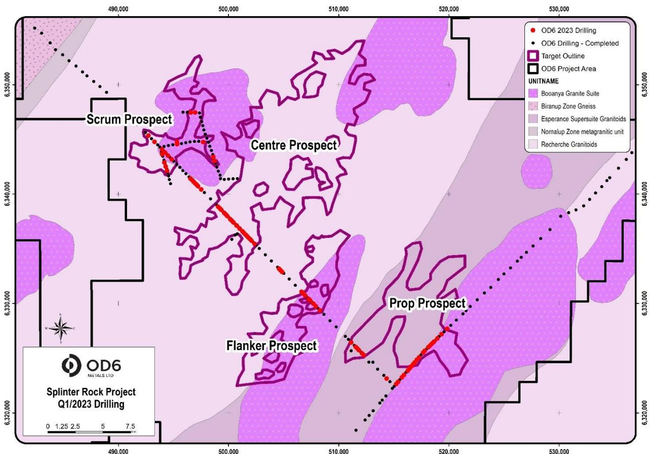
**Figure 3: Splinter Rock geology, prospect and drill locations. Red = Q1/2023 new drilling referred to in this announcement. Black =2022 previous drilling**
