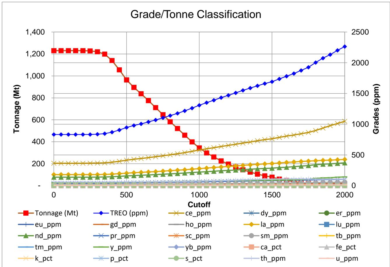
**Figure 1: Splinter Rock Rare Earth project tonnage and grade curve**
