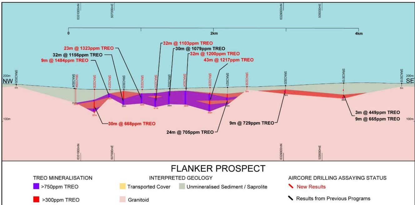
Figure 6: Flanker Prospect Cross Section (vertical exaggeration x6)
