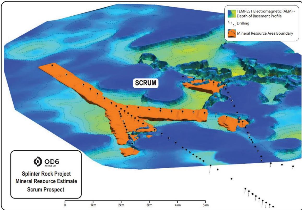
Figure 10: Scrum Mineral Resource interpolation. Oblique view to the north
