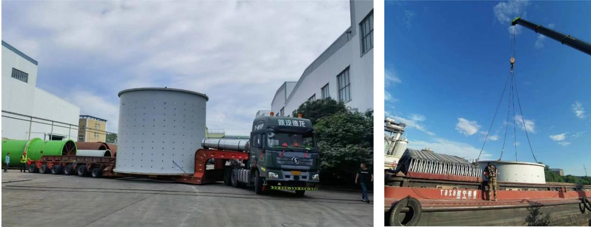
*Figures 5/6: SAG mill shell dispatched by Metso-Outotec*
