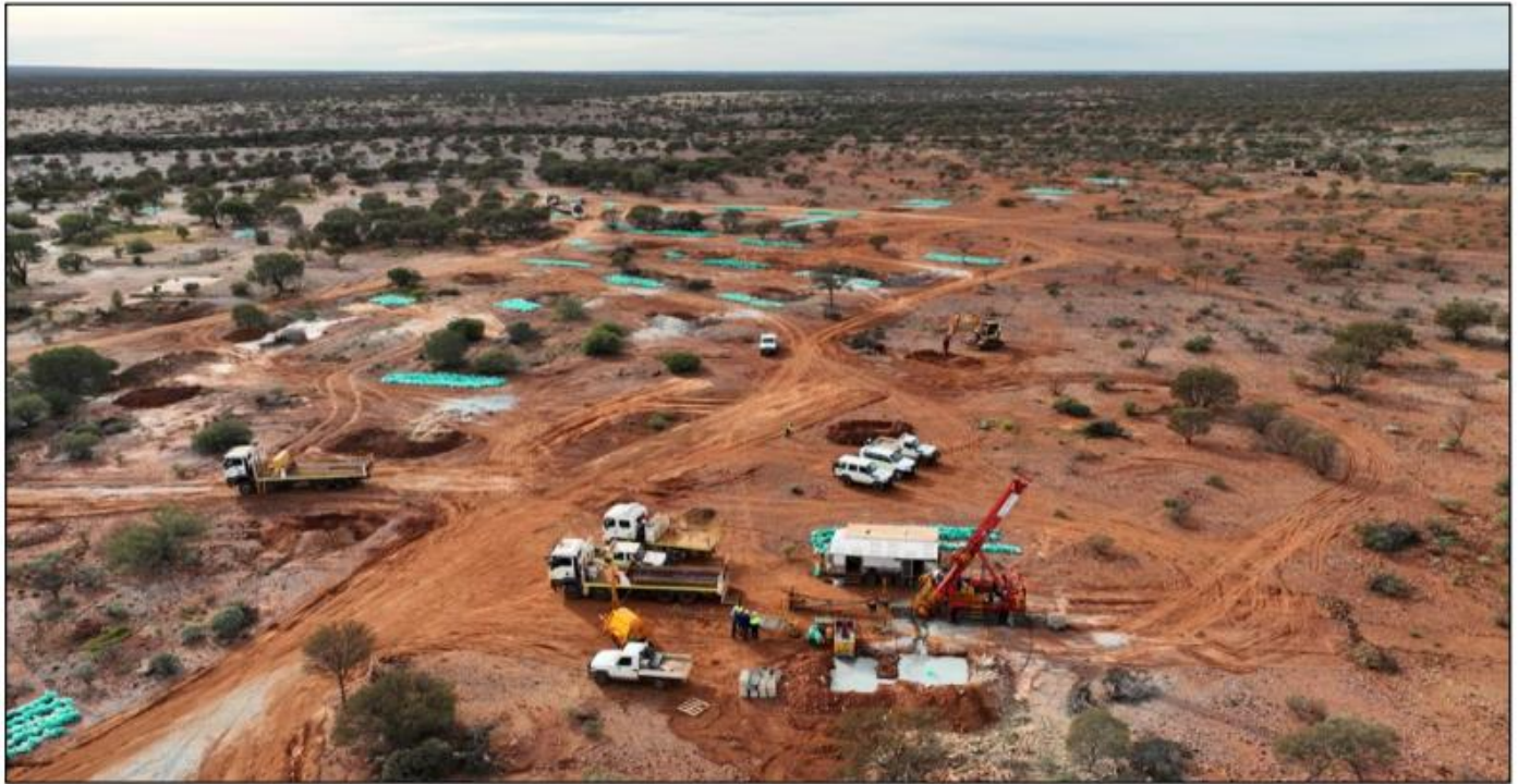
Figure 4. DDH1 Rig 28 Diamond Drilling at Crown Prince Targeting Depth Extensions to Mineralisation (Recent RC pads can be seen in the background along the line of gold mineralisation)
