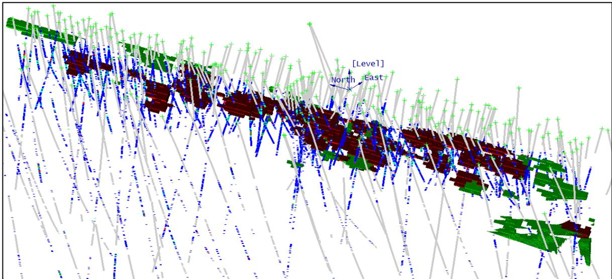
**Figure 10 – Isometric view of Boyd’s Dam looking northeast showing Indicated Resources (red), Inferred Resources (green) and location of drillholes.**
