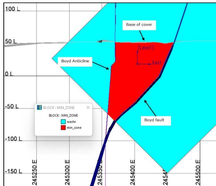
**Figure 9 – Cross section showing the mineralised zone.**
