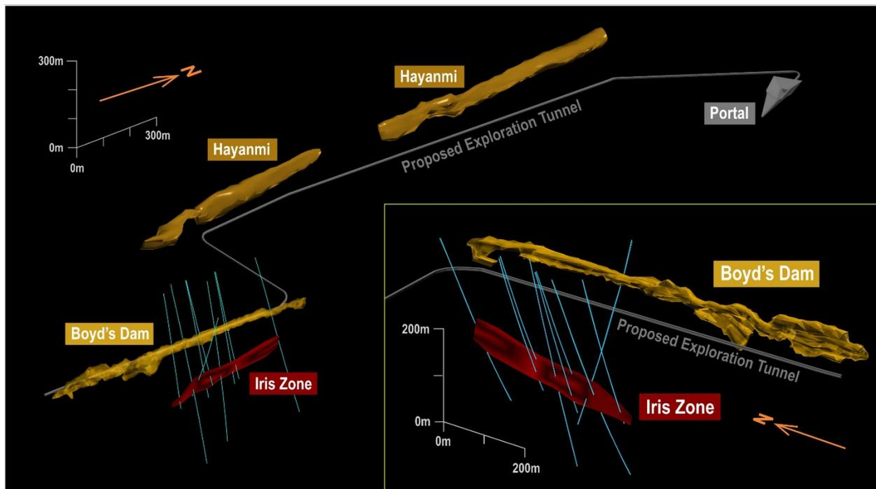
**Figure 7: Four Eagles Isometric view – inset focus on Iris Zone (in red) at depth. Boyd's Dam and Iris Zone represented as their respective alteration zones of sericitic alteration**
