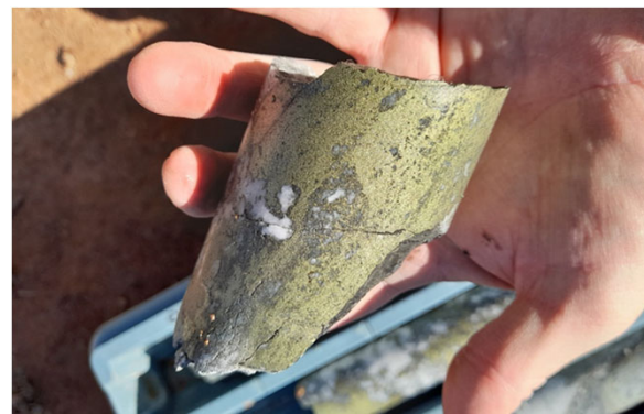
Figure: KSNDDH015 - 71.9m: Chalcopyrite vein. Sample interval 71.6m to 72.3m: 5.5% Cu, 0.5g/t Au, 13g/t Ag.
