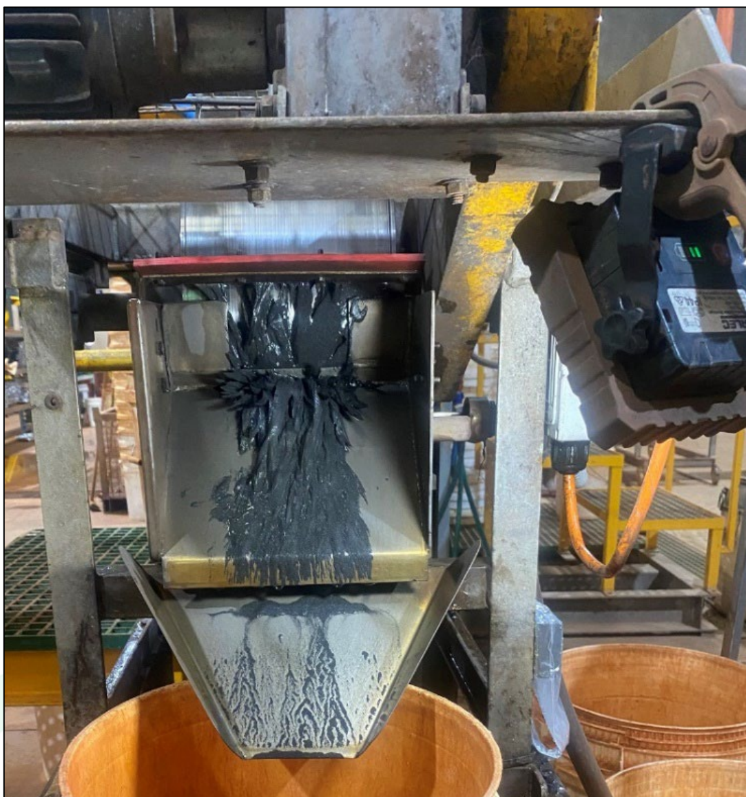
Figure 2. Wet LIMS magnetic separation plant simulation at IOTC Laboratories.
