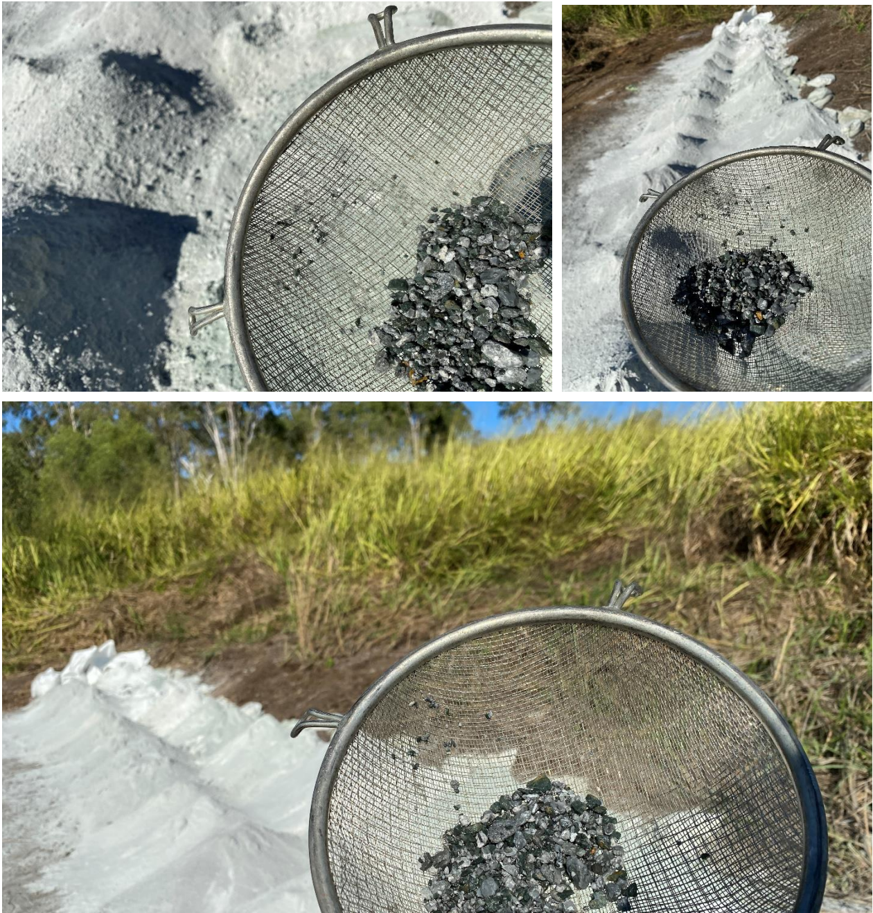
Figure 4: Semi massive sulphides in hole MCRC063 at 49 – 50m.
