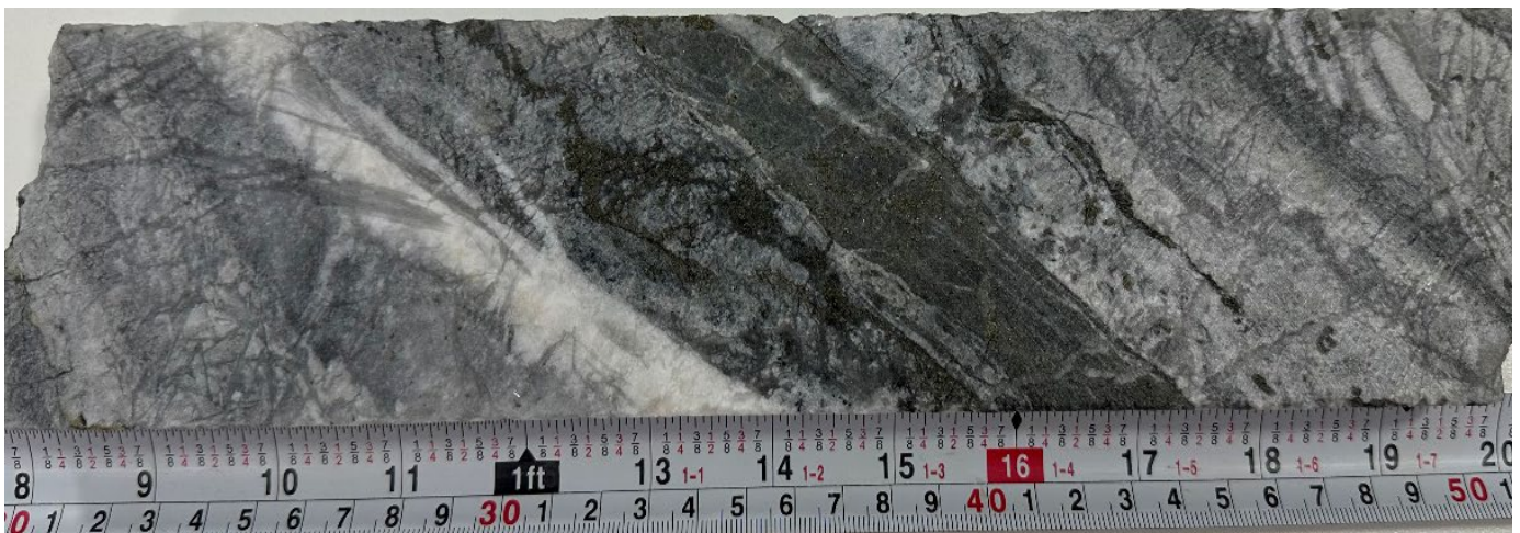
Plate 2: CVDD23-101- 404.6m. Massive epithermal quartz-gypsum-barite-carbonate-pyrite-arsenopyrite-sphalerite vein.
