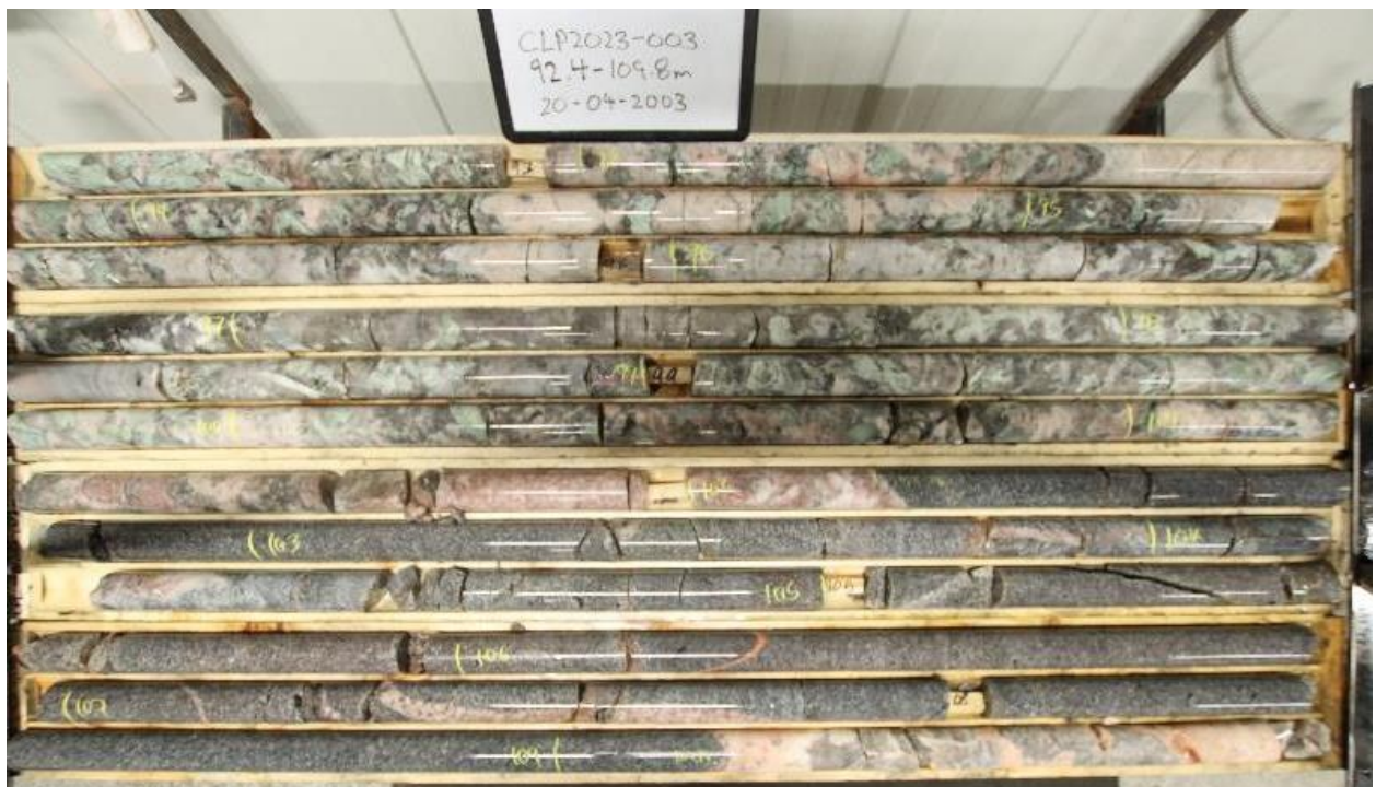
Photo 2. Chubb diamond drill hole CLP003 intersected 9m at 1.34% \text{Li}_2\text{O} of large crystal spodumene-bearing pegmatites from 91m depth.
