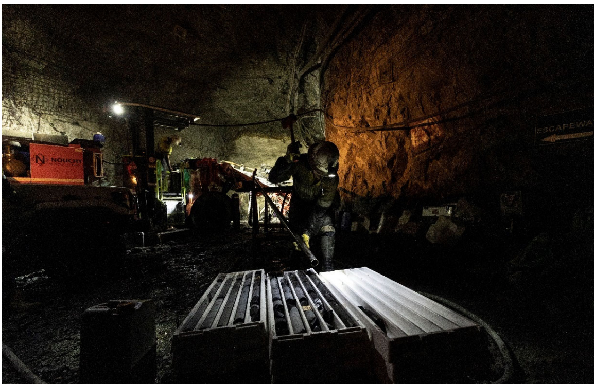
Figure 1: Underground diamond drilling at Paulsens
