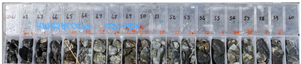
Figure 1. South Hope – chip tray samples from HMHSRC007 between 40 and 60m: 2m at 12.35% Cu and 0.88g/t Au from 46m within 15m at 3.47% Cu and 0.67g/t Au from 44m.
