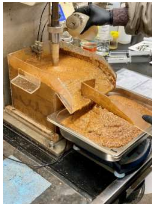
Figure 9: Successful froth flotation test on the Yin bulk sample.
