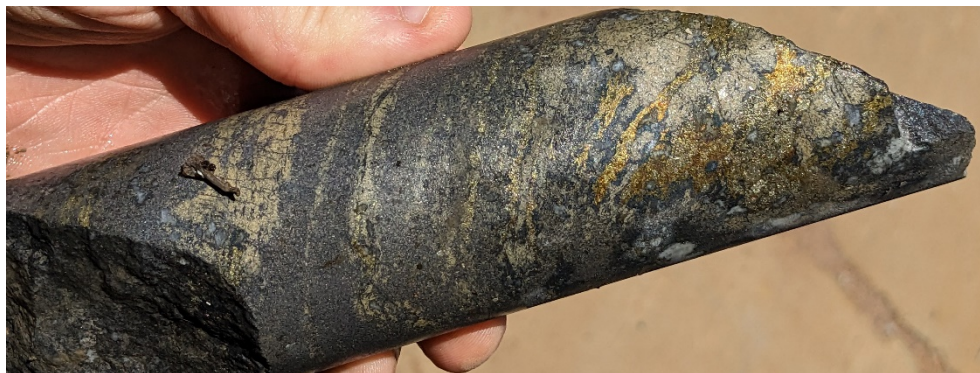
Figure 1: Chalcopyrite, sphalerite & galena mineralisation at 81m in LTDD22080 within an interval of 10.1m @ 12.5% ZnEq. *ZnEq% is an estimate of recoverable zinc equivalent as calculated on Page 8 and in Table 1.
