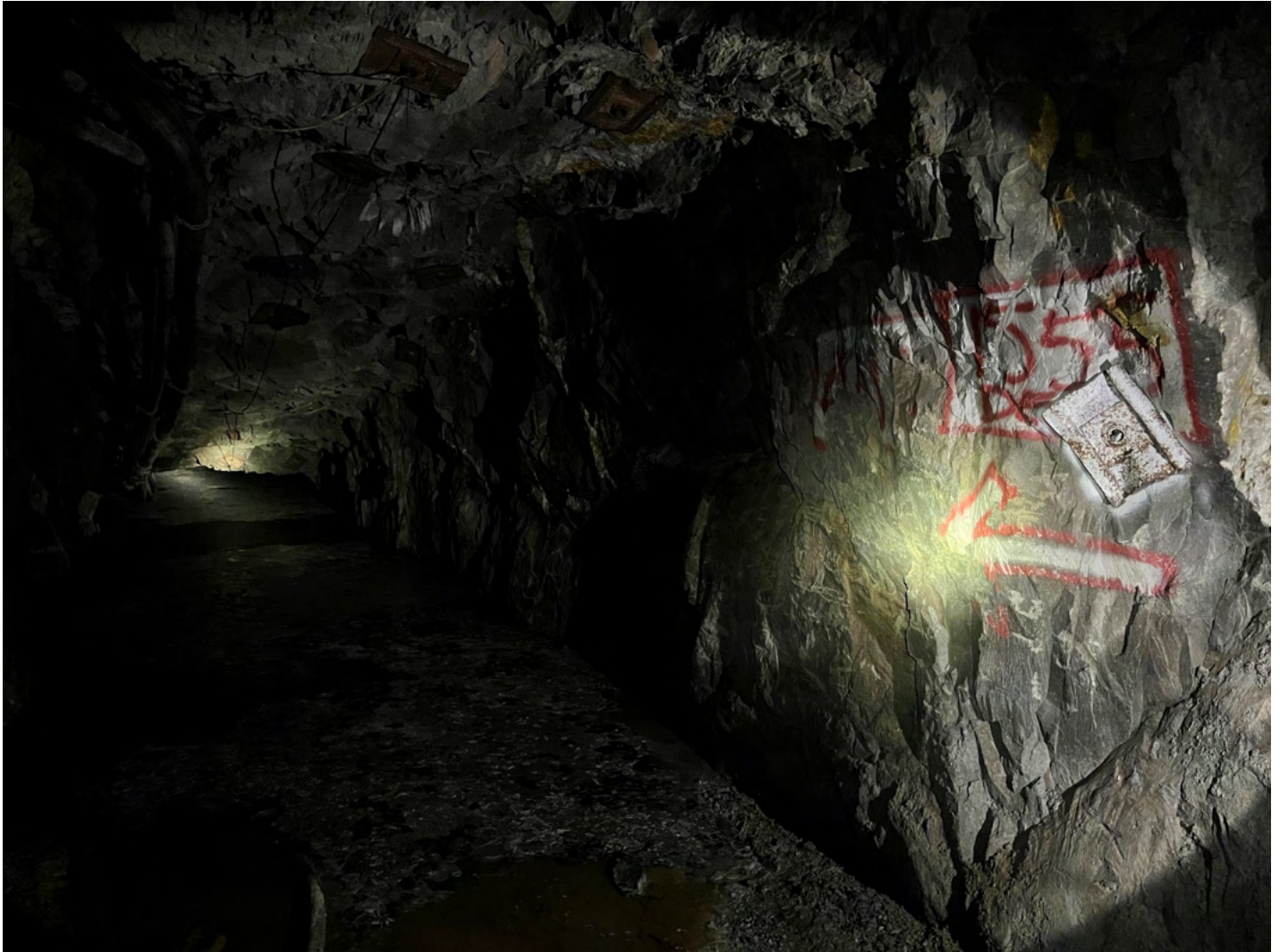
Plate 8. Showing 1555 Decline ready for pumping and re-entry.
