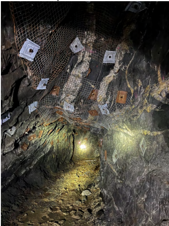
Plate 4. Showing ore drive with partially stripped backs.
