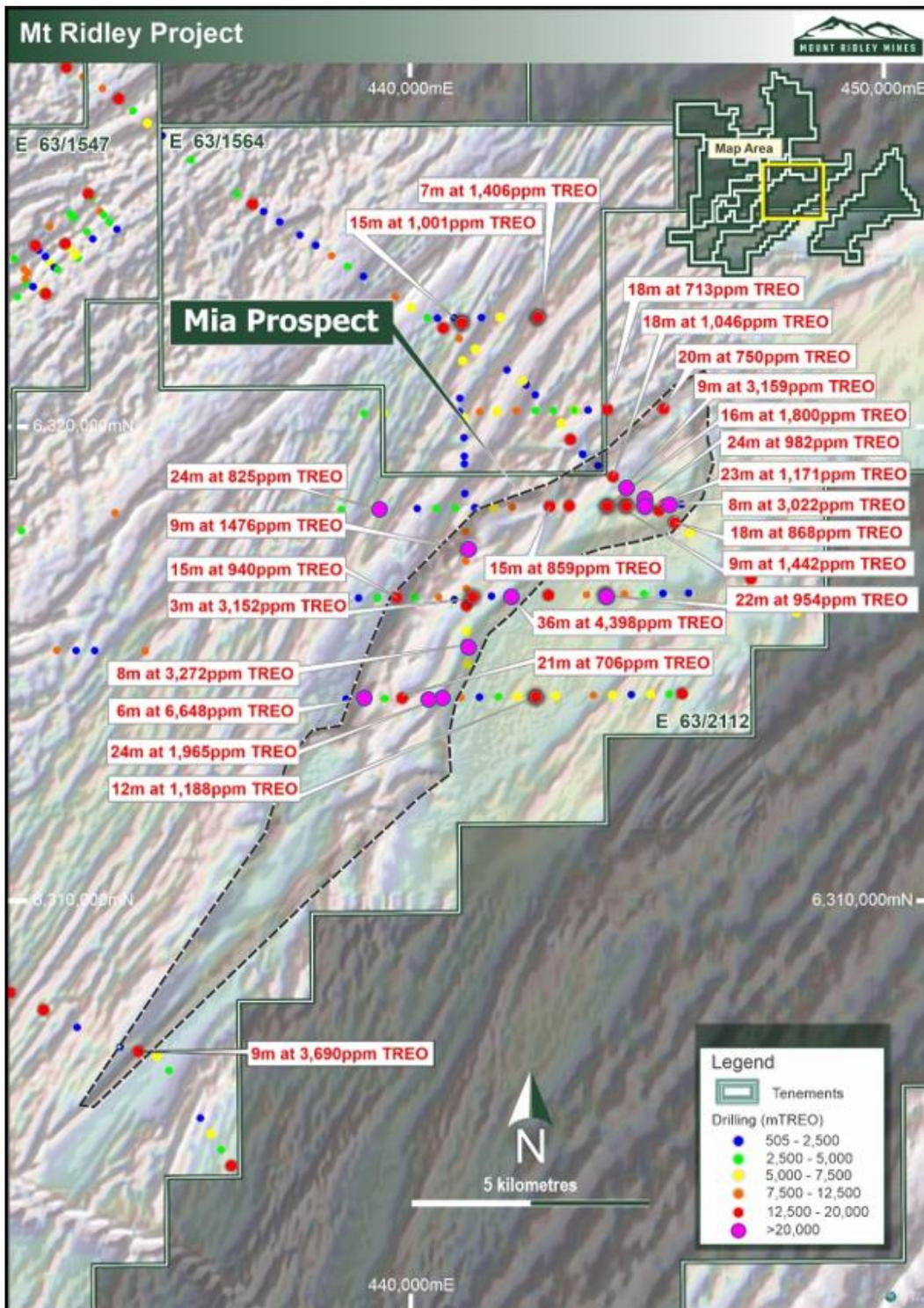
**Figure 2:** Highly enriched REE intersections occur in proximity to a series of parallel, approximately linear, magnetic 'ridges' seen in aeromagnetic imagery over a strike length that exceeds 16 kilometres at the Mia Prospect to date.
