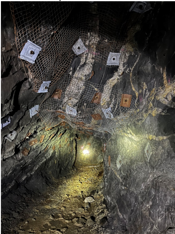
Plate 4. Showing ore drive with partially stripped backs.
