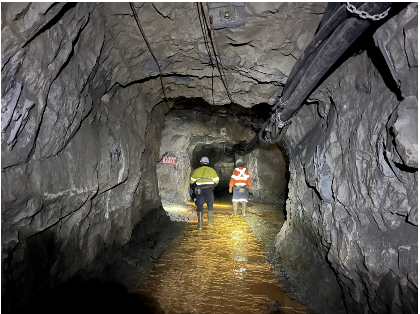
Plate 1. Showing Electrical Contractor Jeff Williams (L) and former underground miner David Thompson (R) in the Amalgamated Adit/640L (NB:- clean floor, good quality ground and service pipes all in very good condition)
