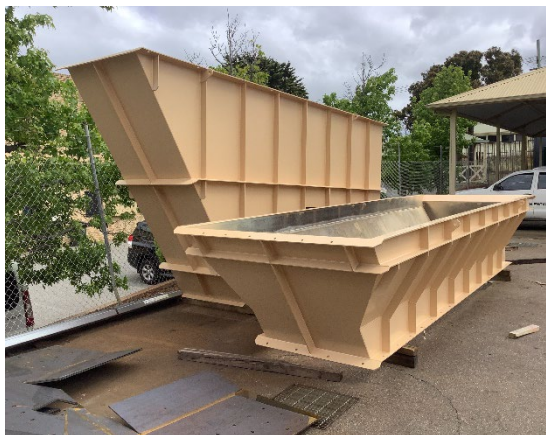
Figures 4-7: Top - Chutes and screens ready for transport to site. Middle – secondary crusher landed in Perth. Bottom - mill fabrication well advanced for delivery to site ahead of schedule in March 2023. Mill fabrication shown in picture.
