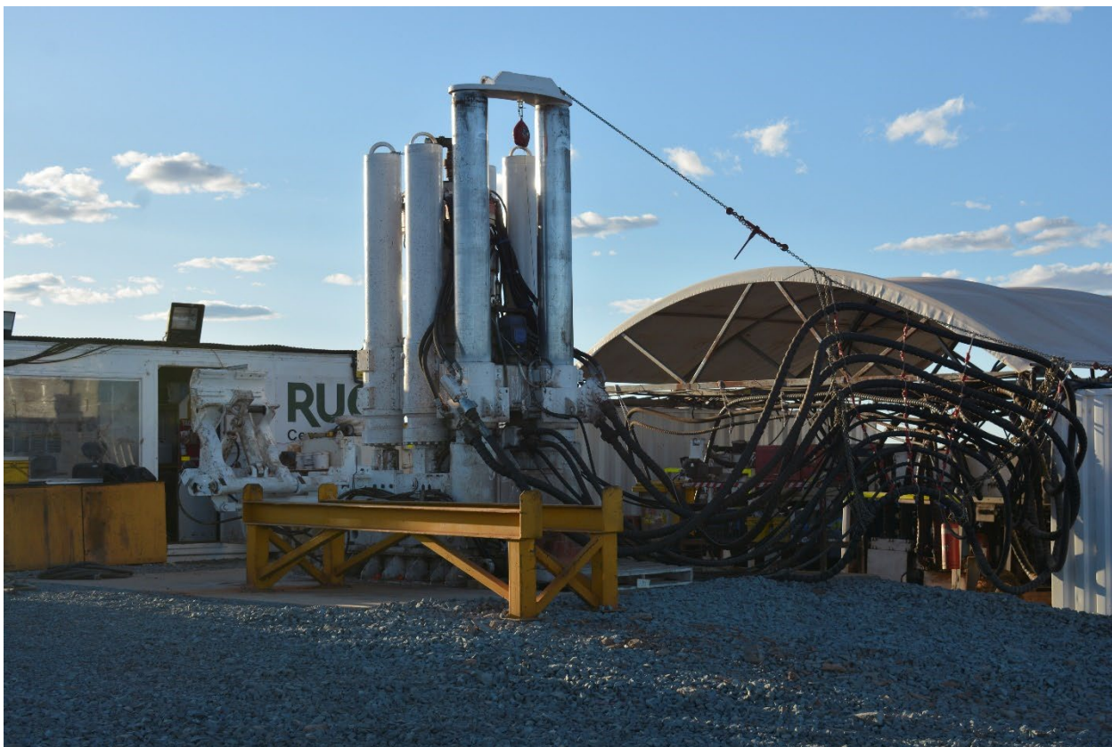
Figure 15: Raisebore set up drilling pilot drill hole for Armand/Marceline escapeway
