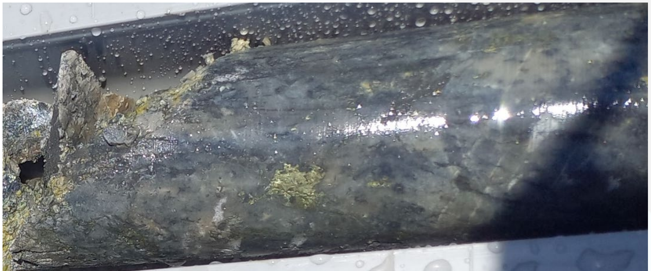
Figure 6. MHDD045 diamond core showing interpreted felsic intrusion host with chalcopyrite from 183.2 – 183.4m.
