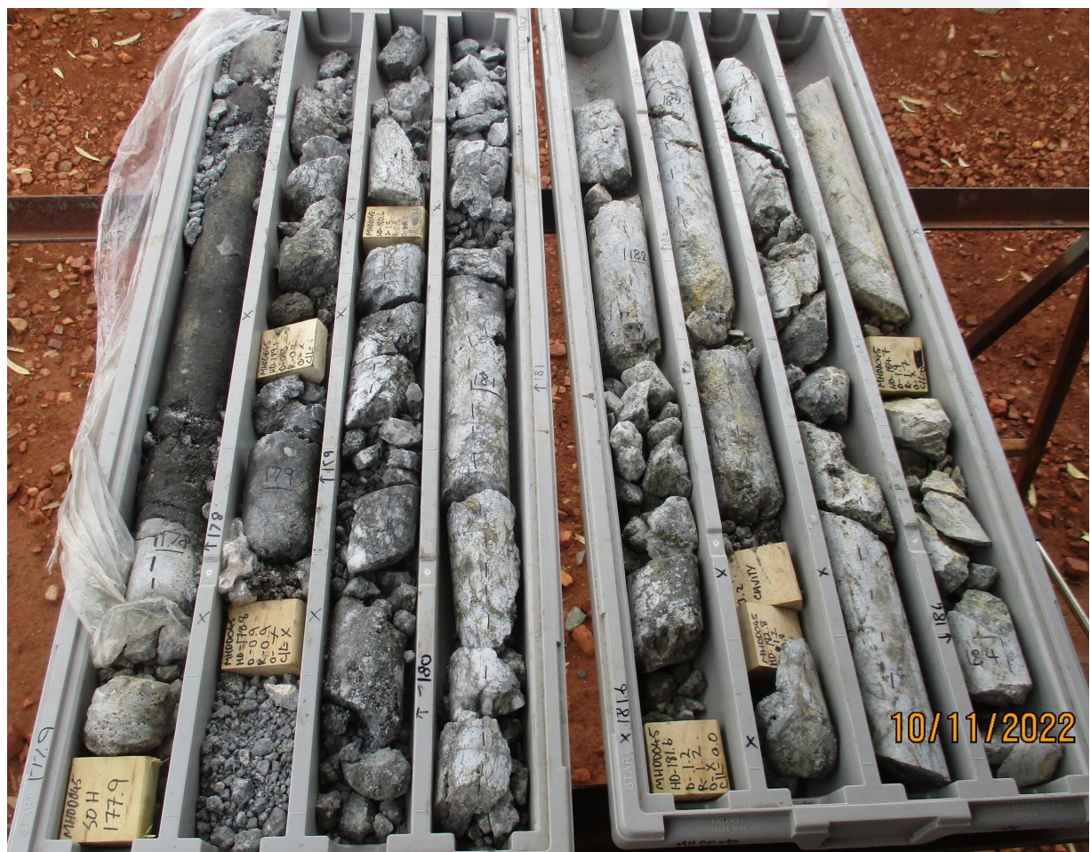
Figure 4. MHDD045 diamond core showing intense chalcocite in fine milled quartz breccia from 178 to 179m and quartz-chalcocite-chalcopyrite breccia after 179m.
