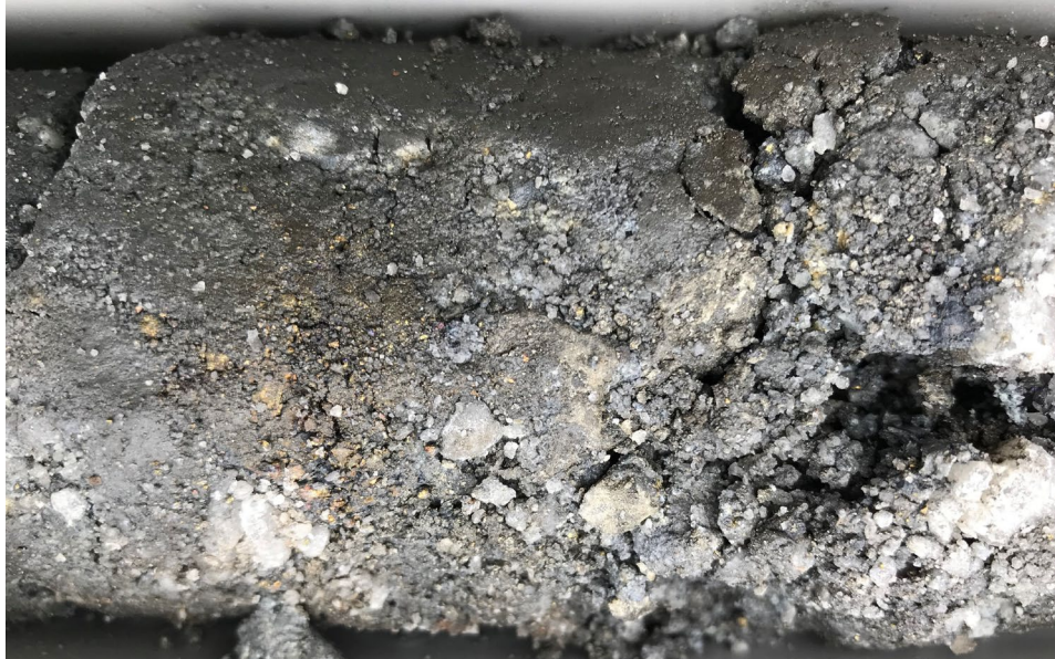
Figure 3. MHDD045 diamond core showing intensely milled quartz chalcocite chalcopyrite breccia zone high grade mineralisation 178.1 – 178.2m.
