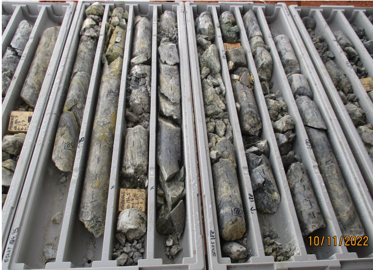
Figure 5. MHDD045 diamond core showing brecciated interpreted felsic intrusion host with chalcopyrite and chalcocite mineralisation.
