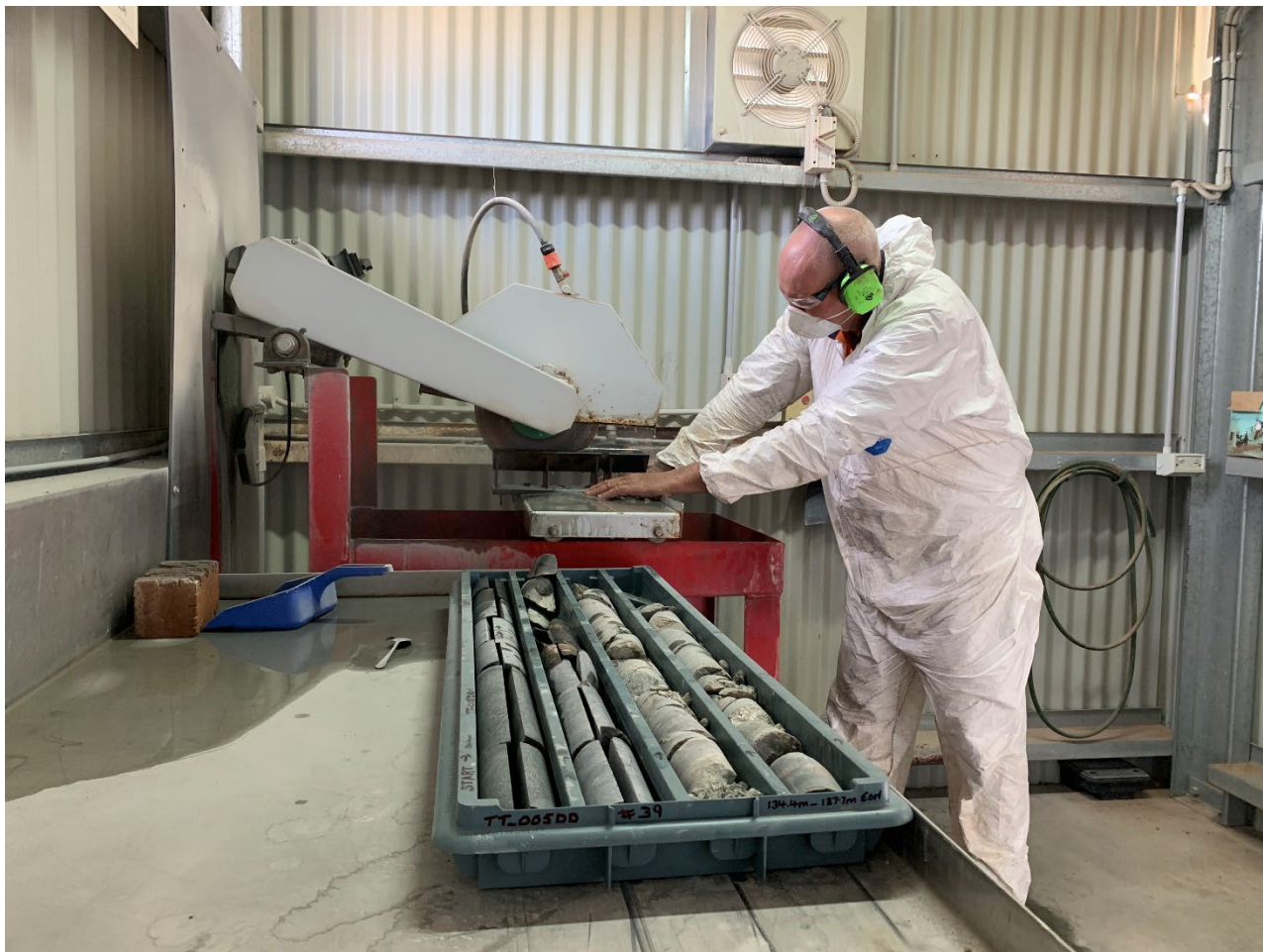
FIGURE 5: CUTTING CORE FROM TT_005DD
