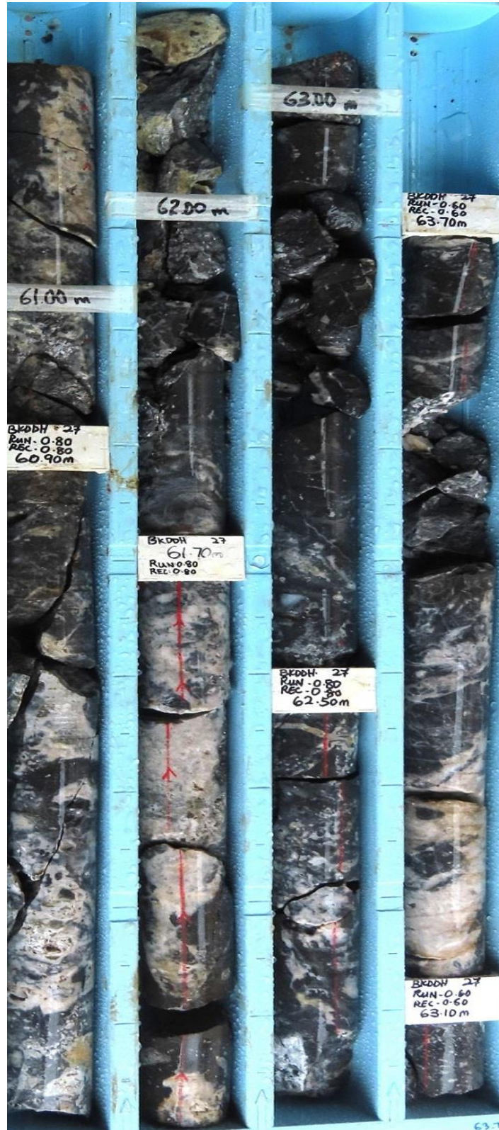
Figure 7: Portion of BKDDH-27 core, between 60.0m-63.7m, illustrating intense alteration in a zone hosting bonanza gold grades: 0.5m @ 209 g/t between 60.5m – 61.0m; 1m @ 64 g/t between 61.0 – 62.0 m; 1 m @ 15.9 g/t between 62.0m – 63.0m & 1m @ 31.8 g/t between 63.0m – 64.0m.
