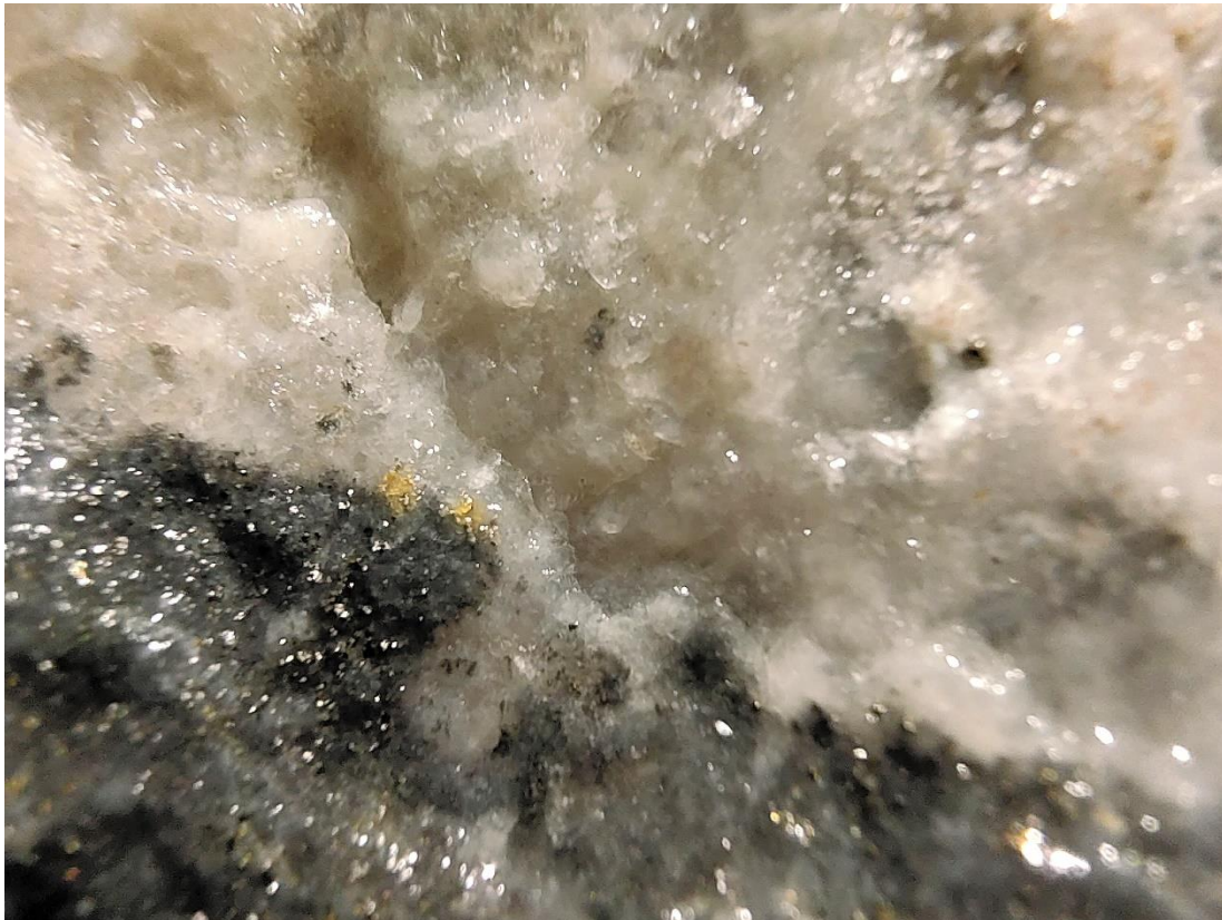
Figure 8: Highly unusual example of free gold in a core sample of BKDDH-27 from the deeper mineralisation zone of the Bau Limestone between 61m-65m.
