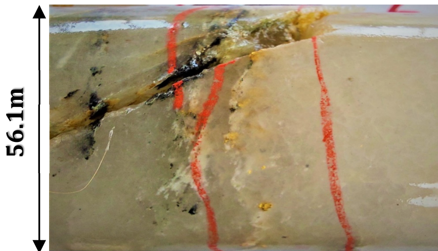
Figure 3: Visible gold in diamond core from ZDD1440 over the interval 61.5m to 62.0m with assay pending
