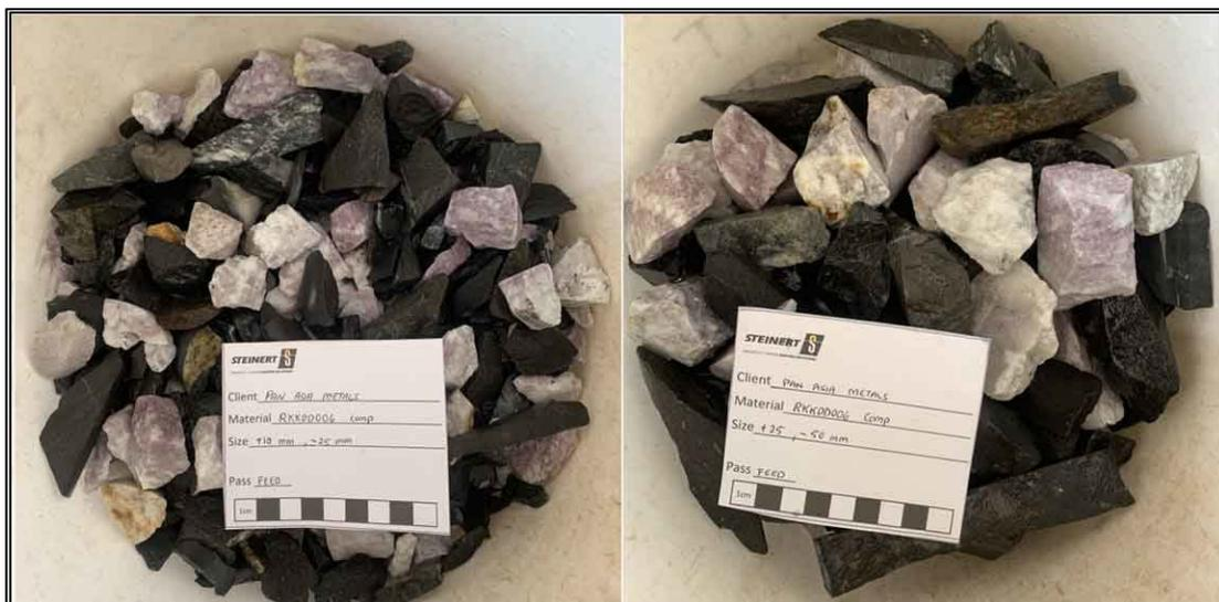
Photo 1. RKDD006: Sub-sample of crushed core feed for ore sorting,
