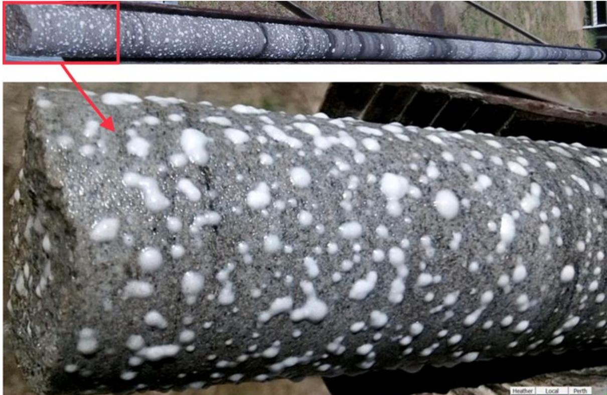
Figure 2- Visible gas emissions from core samples from 270-06C
