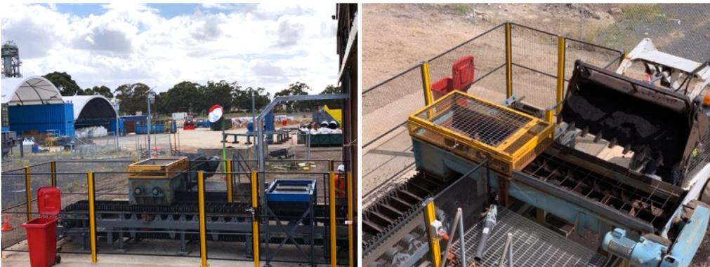
**Above:** Infeed system, where lignite is loaded and conveyed to the hammer mill.
