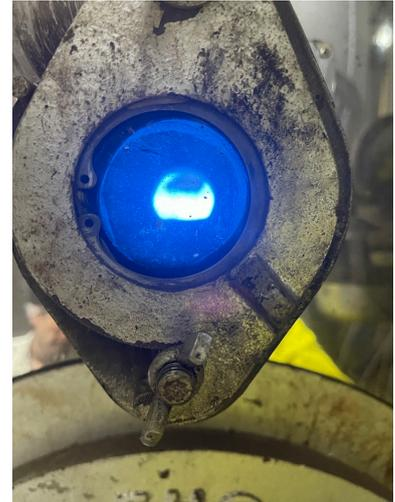
*Above: observation port of the industrial steam system used for COLDry test.*
