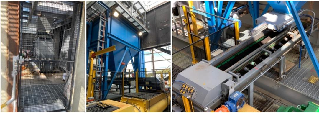
**Above:** hammer mill (left) sizes and screens the lignite before delivery to the surge hopper (centre). The weigh conveyor (right) controls the feed rate into the mixer (below left).
