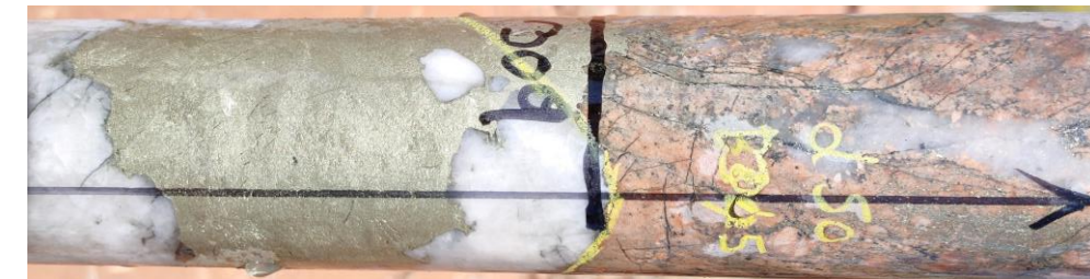
Photo of MHDD024 quart chalcopyrite vein and intense potassic altered host rock with stringer and disseminated Chalcopyrite (Results Pending)
