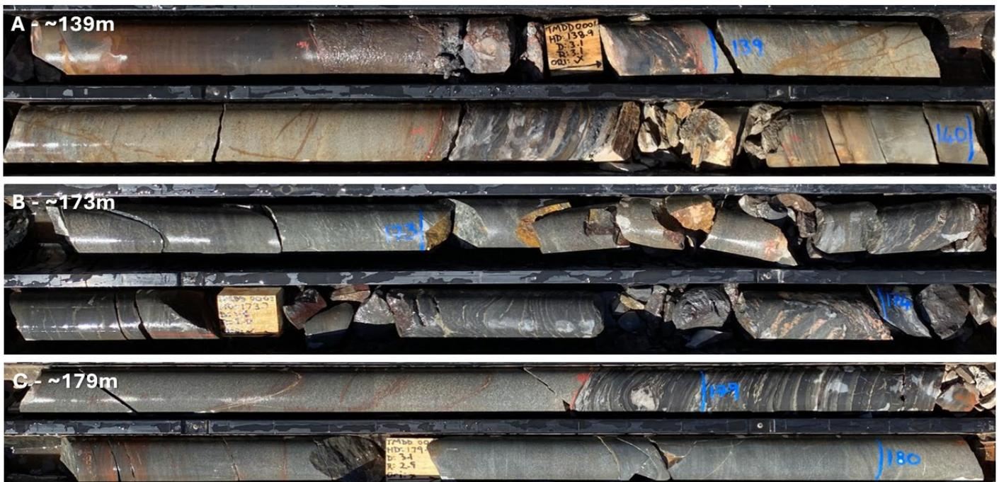
Figure 4. Diamond core photographs of the iron-rich sediments of the Dead Bullock Formation (DBF). A) At approximately 139m, folded iron-rich sediments of the DBF. B) Folded siltstone and shale units of the DBF at ~173m, with multiple folding and shearing events overprinted, with k-feldspar alteration. C) Sediments of the DBF, with increased pyrite and quartz veining.
