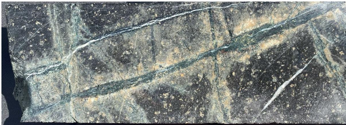
**Figure 3.** Pyrite-chalcopyrite in porphyry-style vein (45.55m-45.85m) part of observed mineralised zone (26m to 49m). PQ core.
