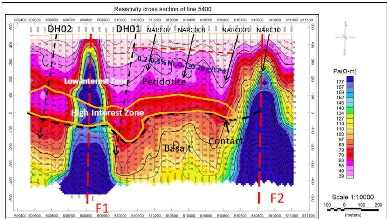
**Figure 3:** Resistivity profile Line 5400 showing the resistive nature of the faults and highlighting the
