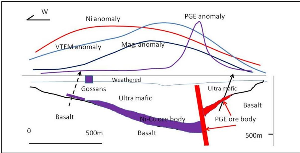
Figure 4: Interpreted geological cross section of Line 5500N
