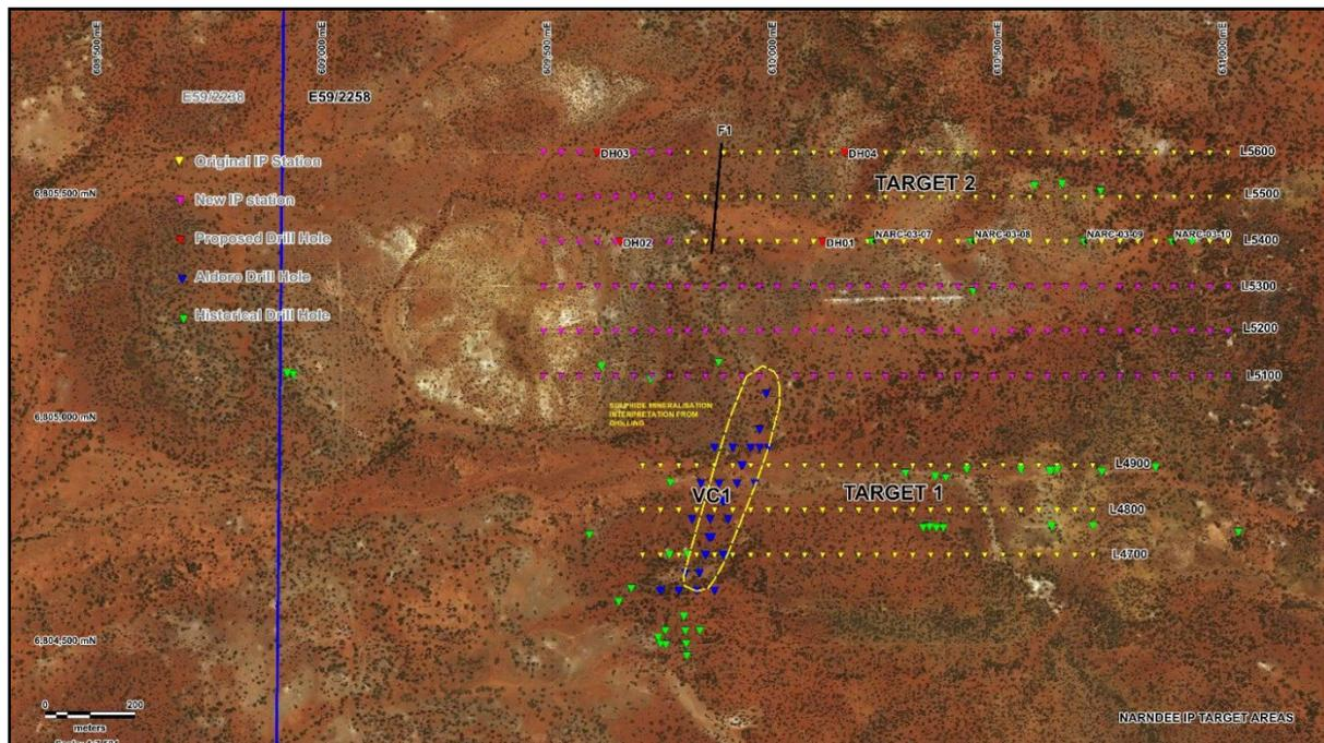
**Figure 1:** Location of the IP survey station/lines, all past drilling, VC1 interpreted mineralisation from drill intersections and the four proposed holes.
