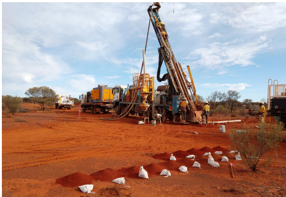
Figure 4: RC drilling at Indomitable.
