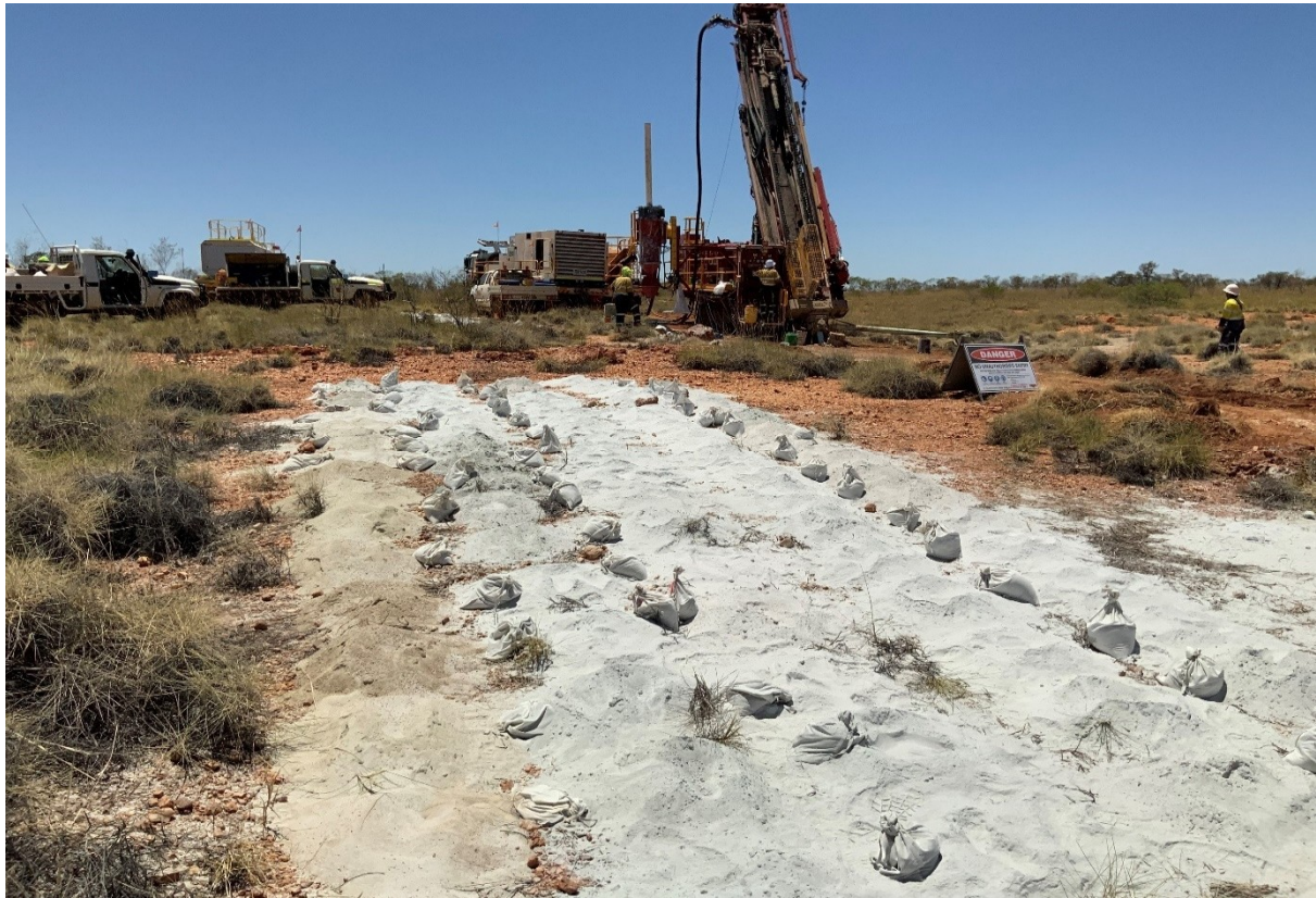
Figure 2 – RC Drilling commenced over North Molyella Project (highlighting pegmatite drill chips on the ground)
