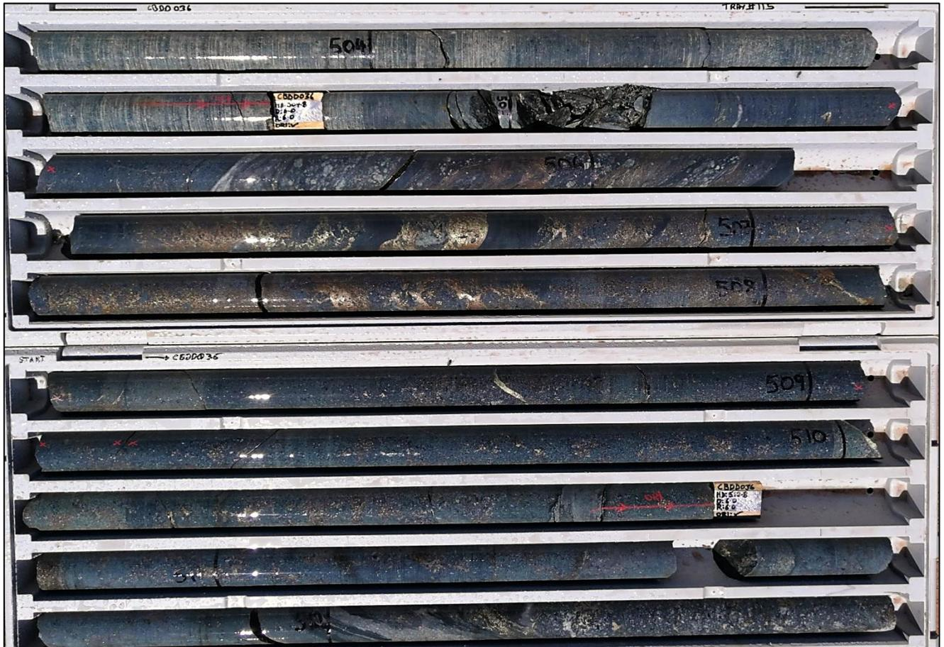
Figure 6. Ni-Cu bearing disseminated, matrix and stringer/vein sulphides within diamond drill hole CBDD036 at the T5 Ni-Cu discovery (503.6m- 512.5m shown).
