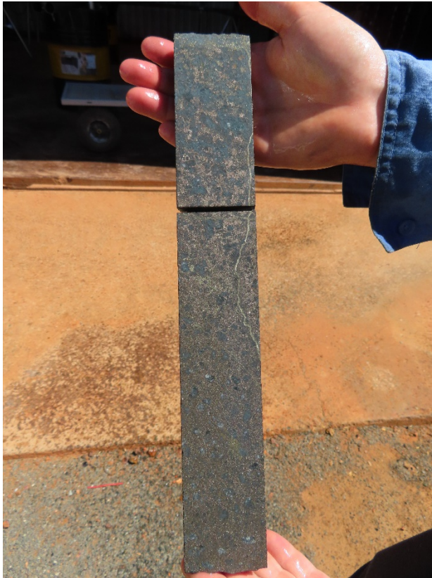
Figure 1: ANDD0007 drill core Matrix to semi-massive to massive Ni-Cu sulphides @ 409.9m – 410.2m
