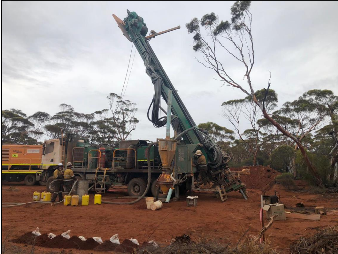
Photograph 1 – RC drilling at one of the regional aeromagnetic targets of the Nepean Nickel Project
