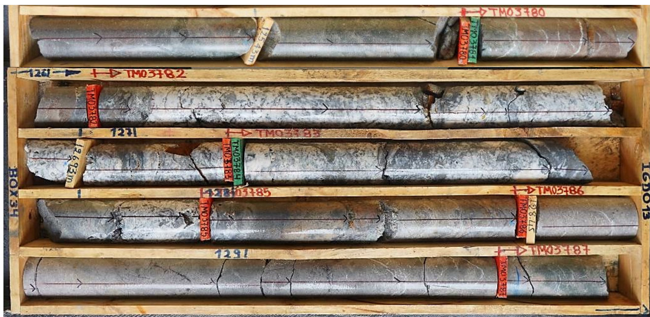
Figure 4: Mineralised intercept from drill hole IGD013, returning 2.69m @ 7.54g/t gold from 125.76m drill depth (image showing recovered core before sampling from 125.1m to ~130.6m depth).
