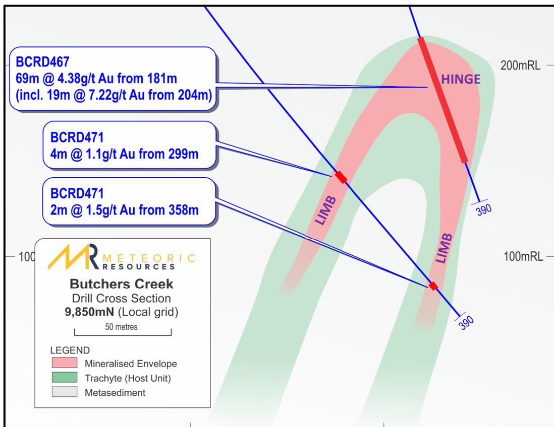
**Figure 3:** A good example (Detail of Section 9,850mN) of the general relationship between thick, robust high-grade intercepts in the Trachyte within the **Fold Hinge** Zone of the fold versus narrower intersections encountered below in the **Fold Limbs**.
