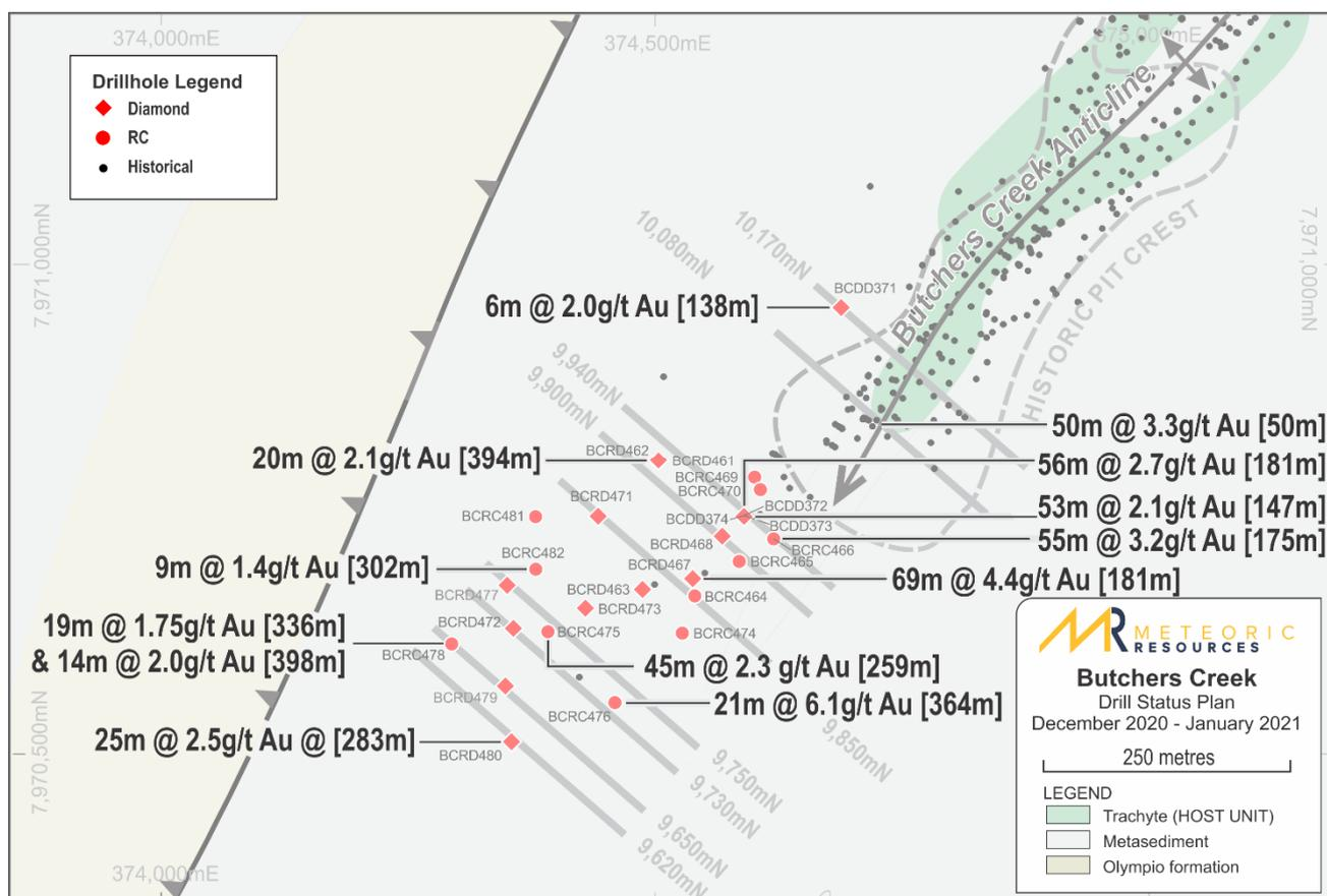
**Figure 1.** Drill hole location plan of 2020 Butchers Creek drill program with Highlight Intercepts from the Company’s 2020 Campaign. Location of all Cross-sections presented in this Release [Figures 3 & 4, Appendix 2] are also shown.
