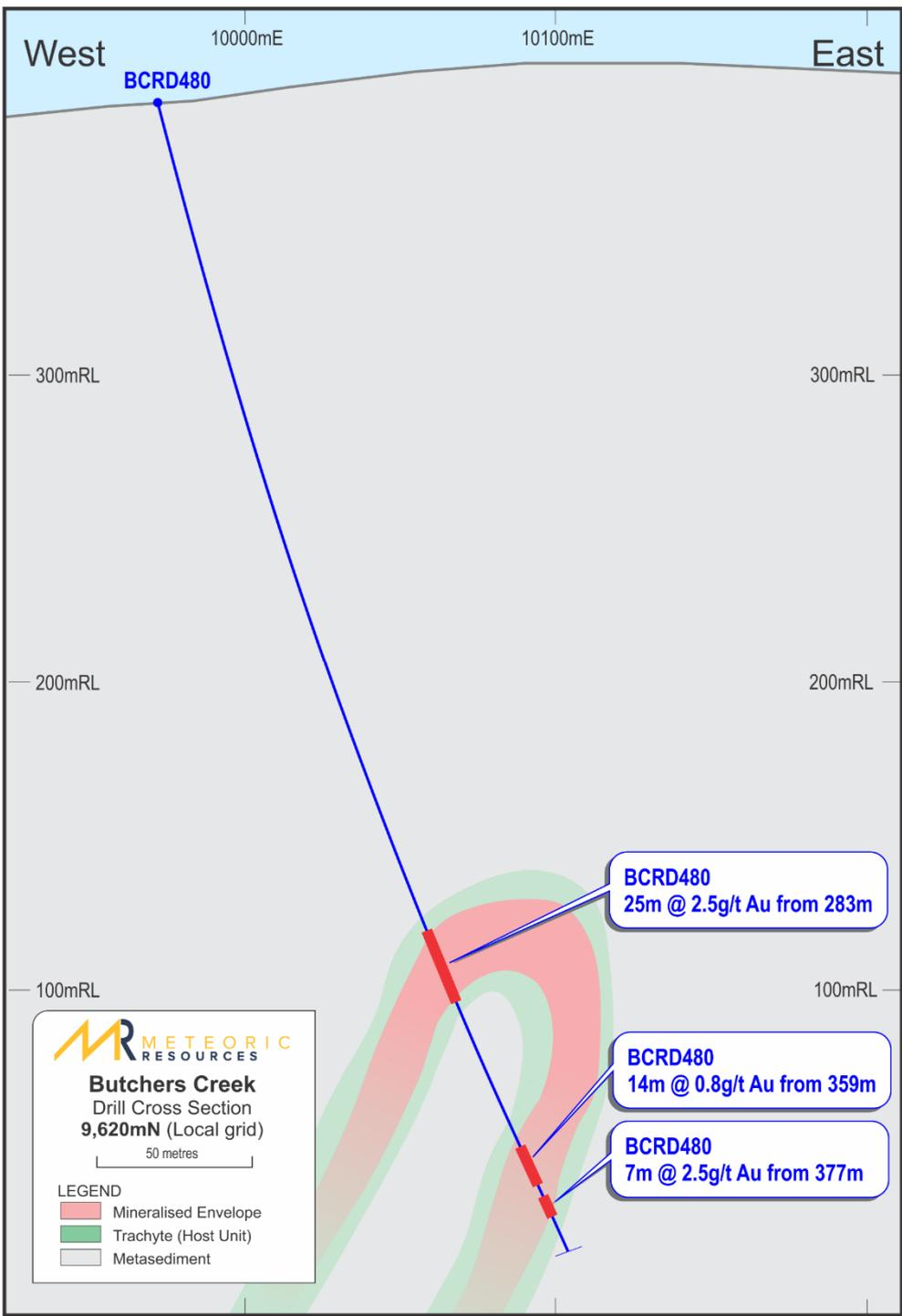
**Figure 6.** Section 9,620mN, 360m south-west of Butchers Creek Open-pit. Visible gold grains were intersected in BCRD480 (380.5m) in 15mm thick quartz-carbonate-chlorite vein with pyrite and pyrrhotite grading 11.05g/t Au (refer ASX release 30 November 2020). Follow up drilling will target thicker, medium-high grade intercepts in the Hinge zone (as observed on other Sections).
