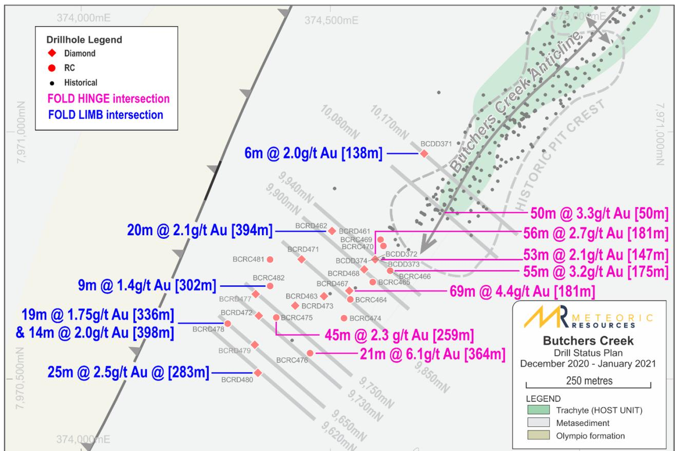
**Figure 2.** Drill hole location plan of 2020 Butchers Creek drill program with Highlight Intercepts from the Company's 2020 Campaign. Note the thicker, higher grade nature of the Fold Hinge intercepts in Purple versus the Fold Limb Intersections in Blue. Location of all Cross-sections presented in this Release [Figures 3 & 4, Appendix 2] are also shown.
