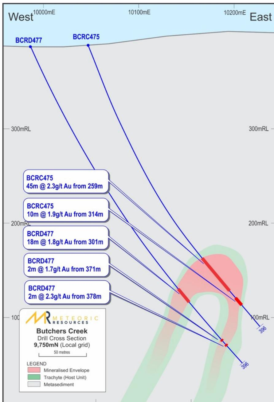
**Figure 5.** Section 9,750mN, 220m south-west of Butchers Creek Open-pit. Visible gold grains were intersected in BCRD477 in a thick interval of mineralisation on the Limb of the fold (18m @ 1.8g/t Au).
