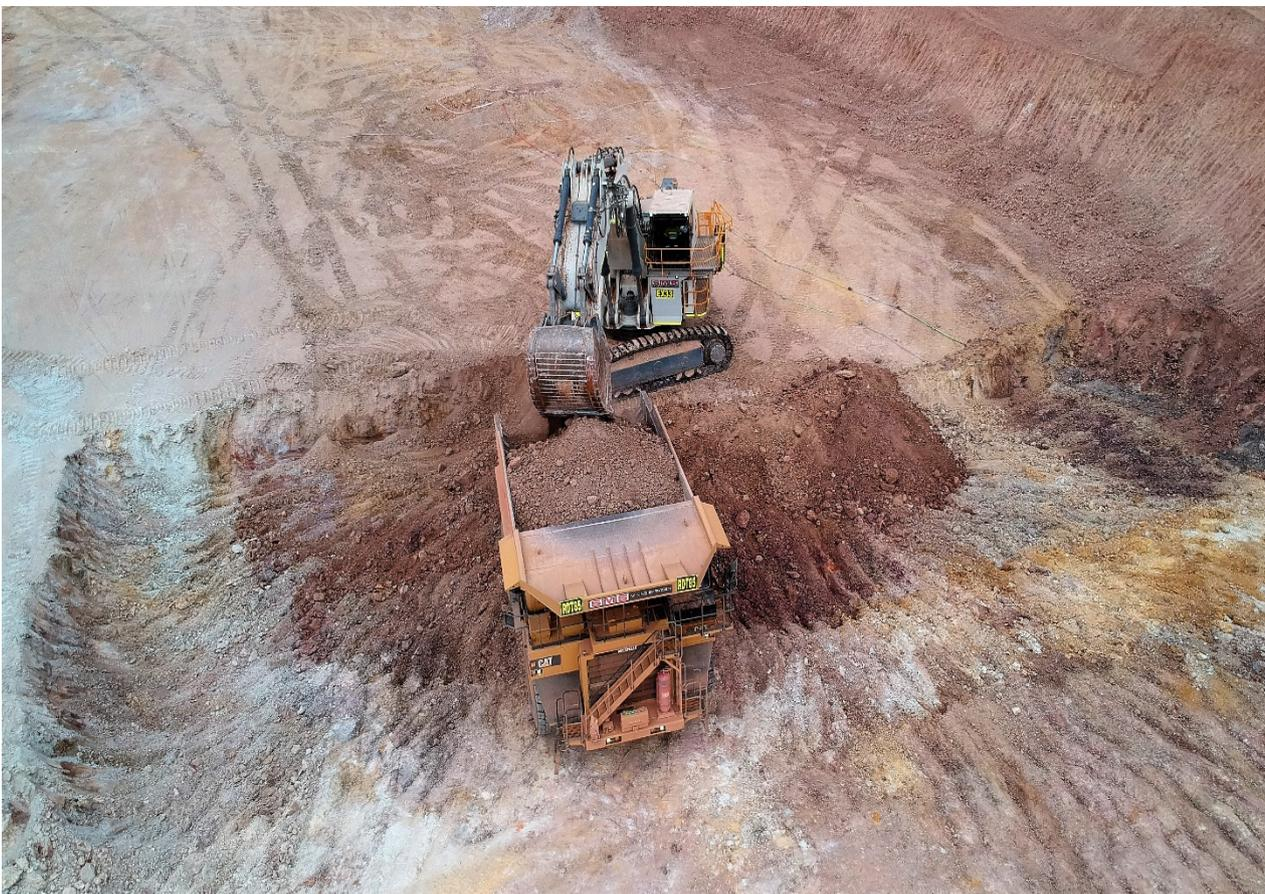
*Figure 8 – 200t excavator at work in the Riverina Open Pit*
