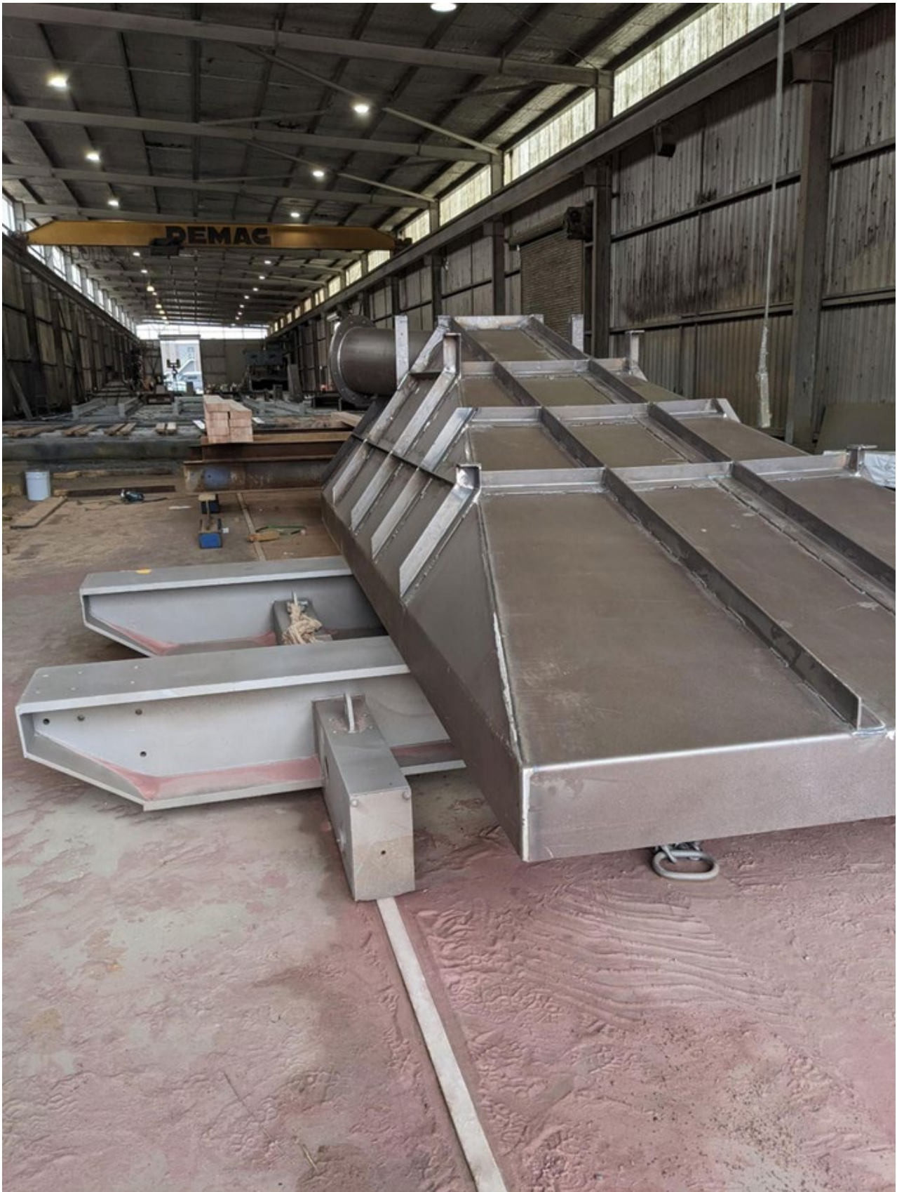
Figure 2 | The Plant's Hopper being fabricated at Crisp Bros & Haywards workshop
