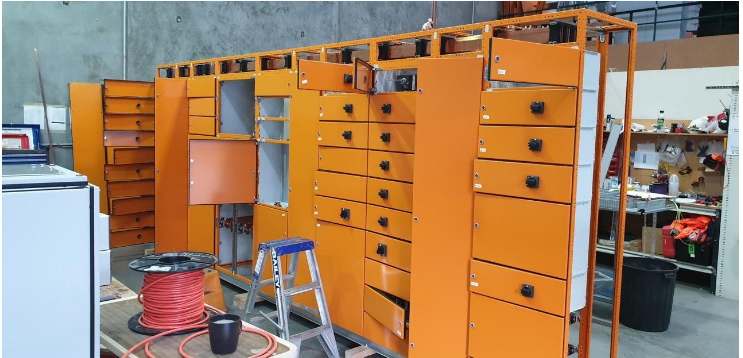
Figure 3 | The MCC being assembled at Tritec Electrical Controls & Automation workshop
