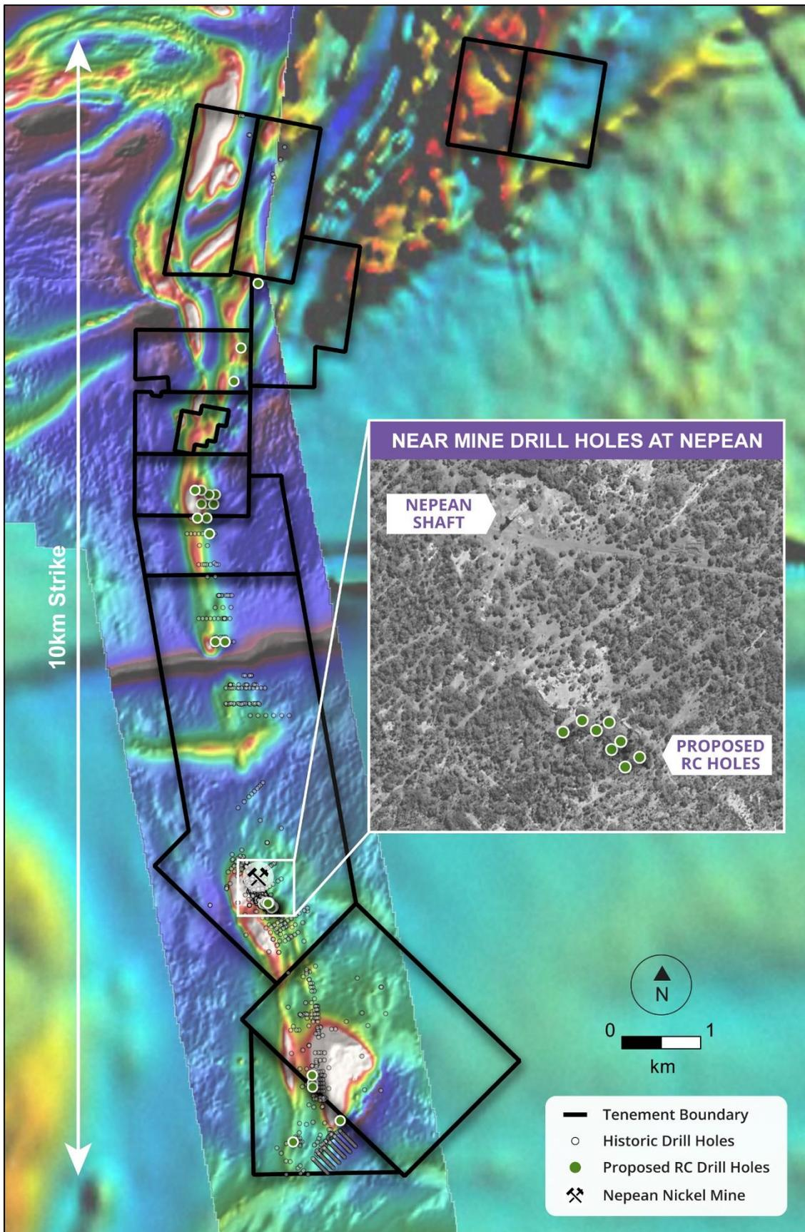
Figure 1 – Plan map of the Nepean Nickel Project showing planned and existing drill-hole collars (RC & DD) relative to aeromagnetic (RTP) highs (high-resolution aeromagnetic survey overlying GSWA 250k merged mosaic)
