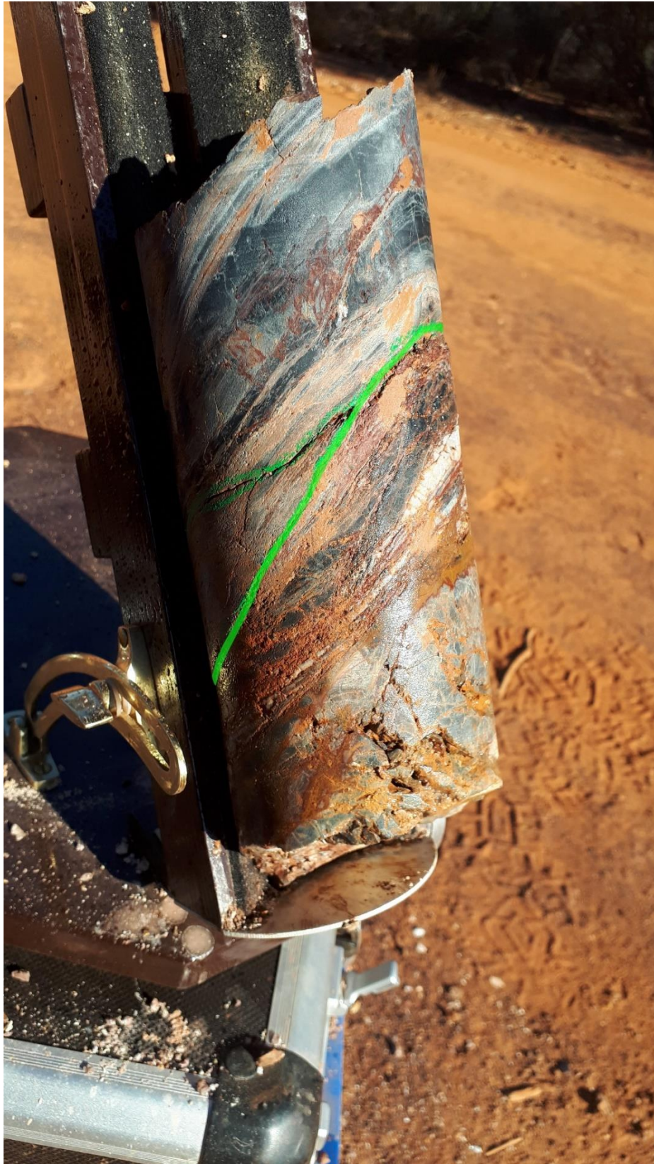
Figure 4: Fault (green line) at 43.0m in SSMH0101
