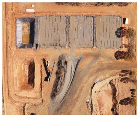
Plan view of the three heap leach pads, pre-stacked scats, with the aeration piping and PLS collection pond (LHS)
