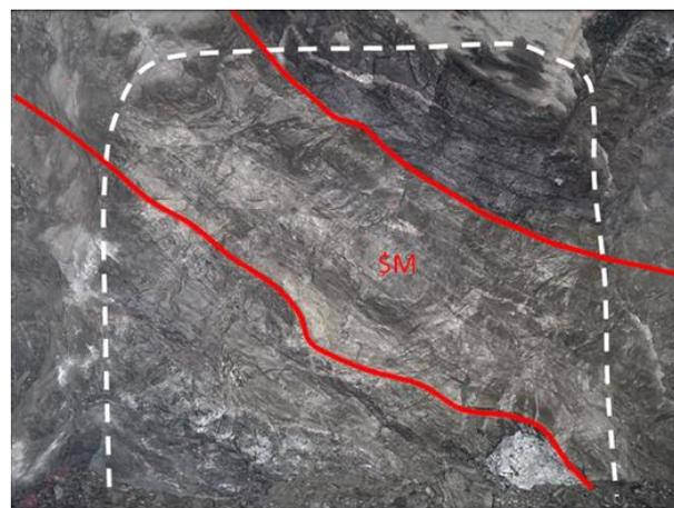
SBA 836 ore drive (3.5 m W x 3.5m H) with a face grade of 5.4% Ni TBA 415 ore drive (4.5m W x 4.5m H) with a face grade of 4.0% Ni
