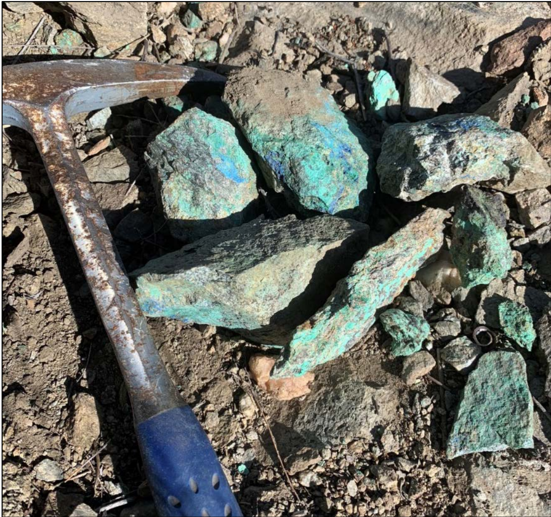
Figure 7 - High-grade waste from dump material at OREX target assaying 9.15% Cu, 192 g/t Ag and 0.15 g/t Au. The sample was collected next to a small adit mined along a copper-bearing shear within the Leatherwood intrusive.
