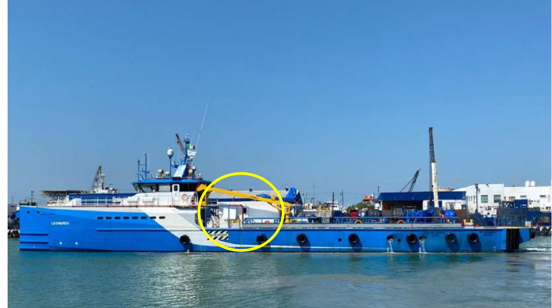
The MV Leonardo with the VG1000SD VEEM Gyro installed on the deck (below the yellow crane boom) ahead of sea trials. Anecdotally, Damen representatives and crew on board during the trials were very impressed with the vessel comfort and performance when the VEEM Gyro was turned on.
